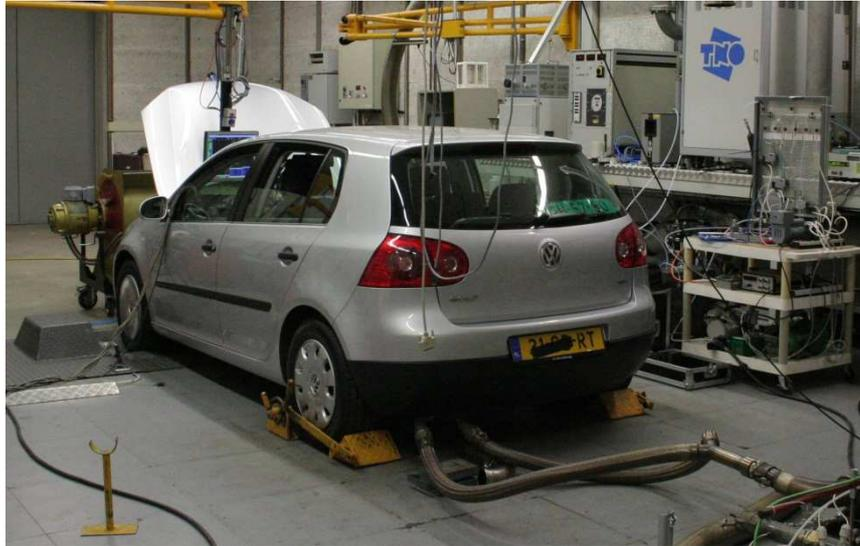
Figure 5: Chassis dynamometer or roller bench
