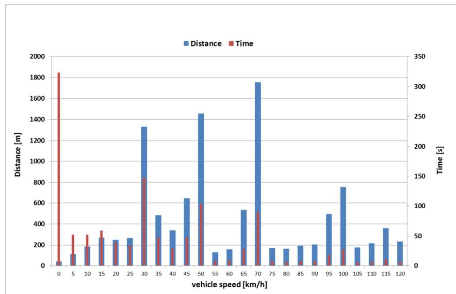
Figure 13: The distribution of distance and time over each velocities in the NEDC test
