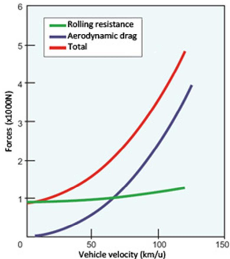
Figure 4: Characteristics of rolling resistance and aerodynamic drag of a vehicle
