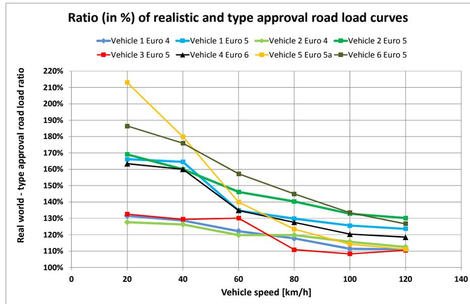
Figure 1: Ratio of realistic and Type Approval road load test results of all tested vehicles
