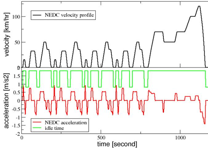
Figure 12: The velocity, acceleration, and idle times of the NEDC test
