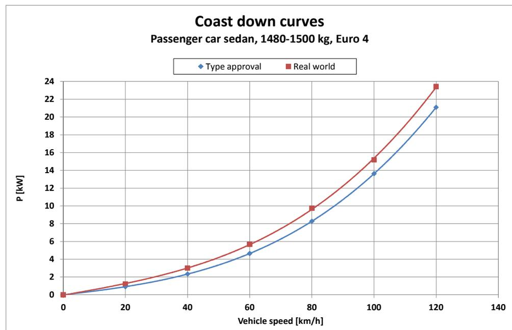
Figure 15: Type Approval and realistic road load curve of vehicle 1 (my 2008)
