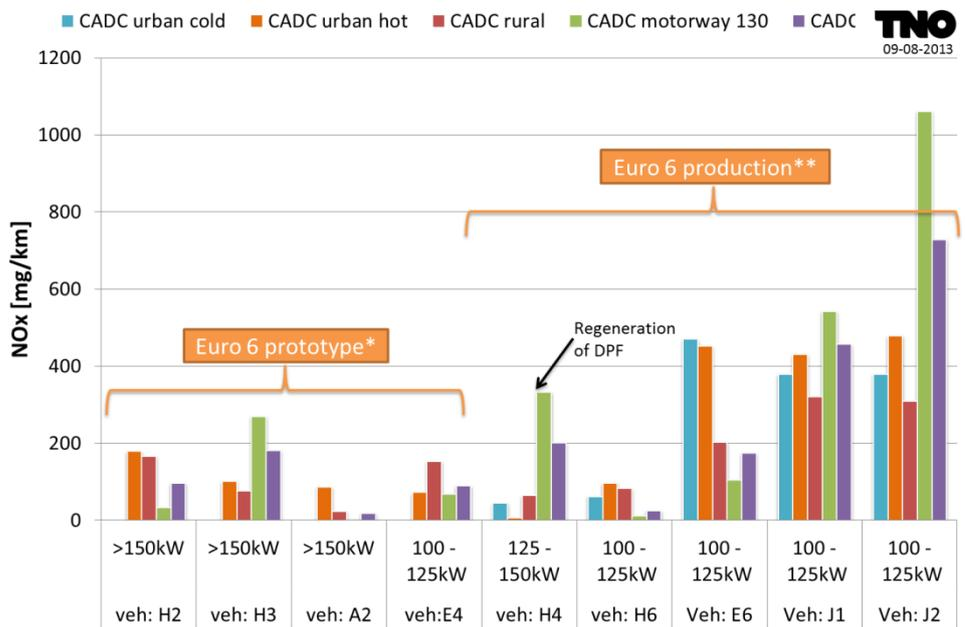
Figure 16: NO<sub>x</sub> emissions per phase in the CADC
