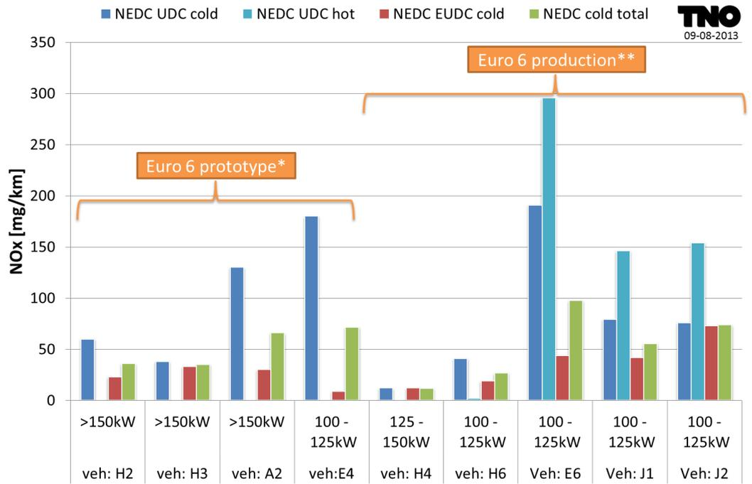
Figure 15: NO<sub>x</sub> emissions per phase in the NEDC
