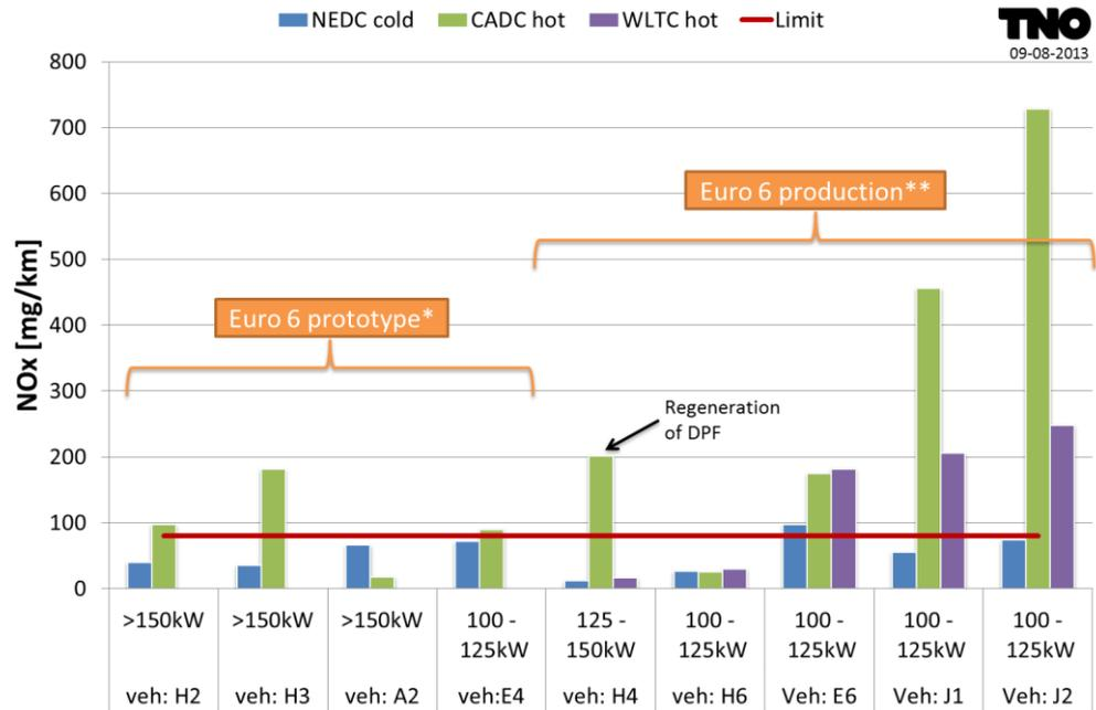
Figure 14: NO<sub>x</sub> emissions per driving cycle
