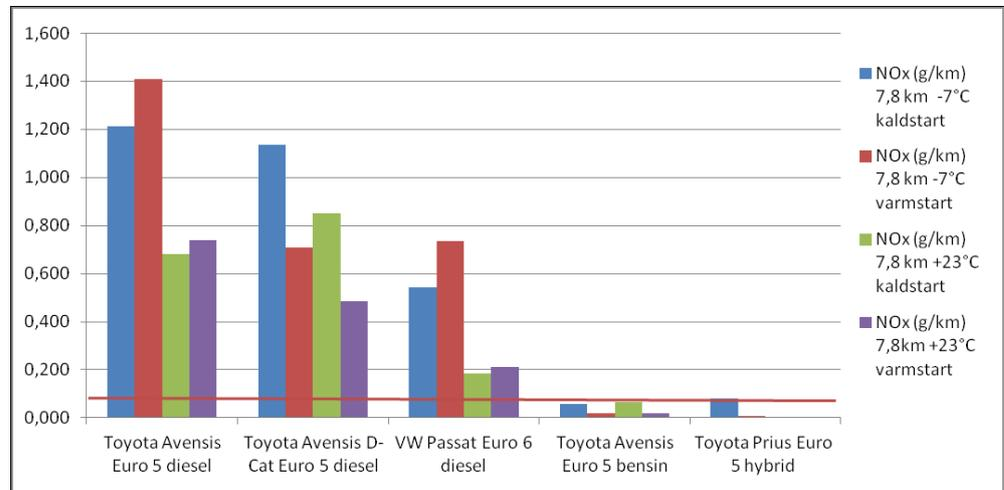
Figure 7: Emissions of NO<sub>x</sub> from six light vehicles tested with the Helsinki city cycle at -7°C and +23°C with cold and warm engine start (Source: TOI-Norway)
