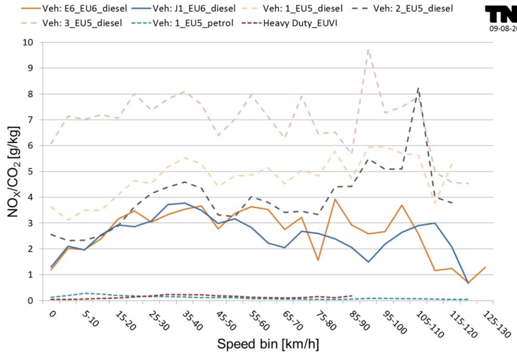
Figure 19: PEMS results binned in NO<sub>x</sub> over CO<sub>2</sub>
