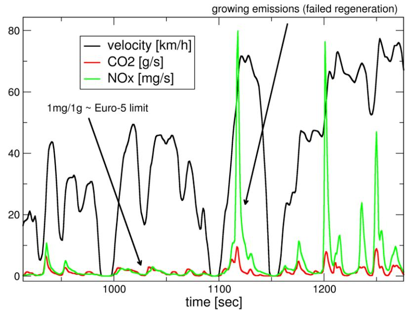
Figure 24 During rural driving NO<sub>x</sub> emissions may grow occasionally due the delayed or failed regeneration of the trap.
