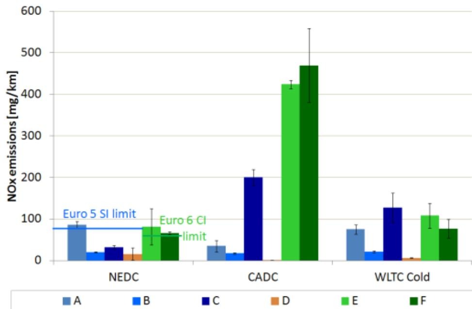
Figure 8: NO<sub>x</sub> emissions @ ambient temperature 25 °C (Source AECC)
