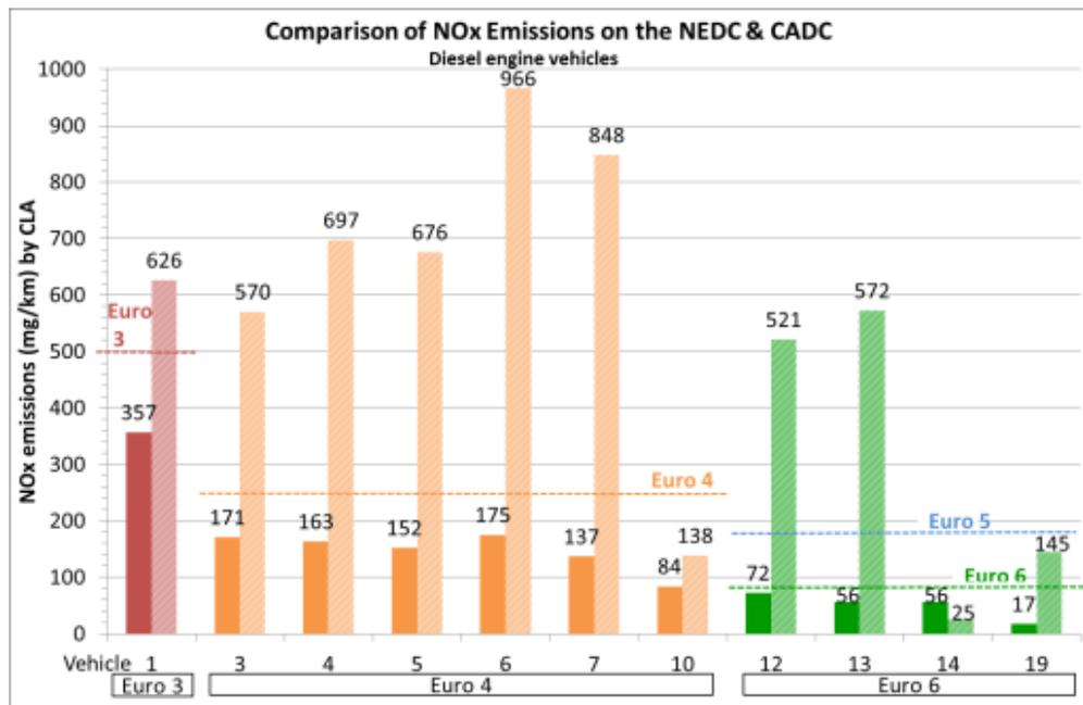
Figure 13: Diesel NOx results over full NEDC and CADC tests (Source AECC)
