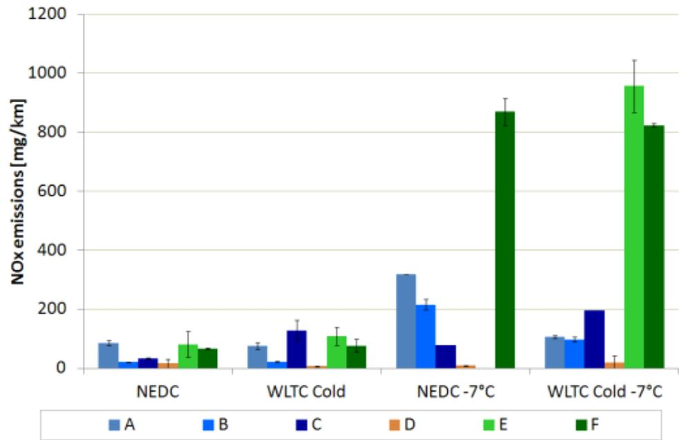
Figure 9: NO<sub>x</sub> emissions at 25°C and -7°C on NEDC and CADC (Source AECC)
