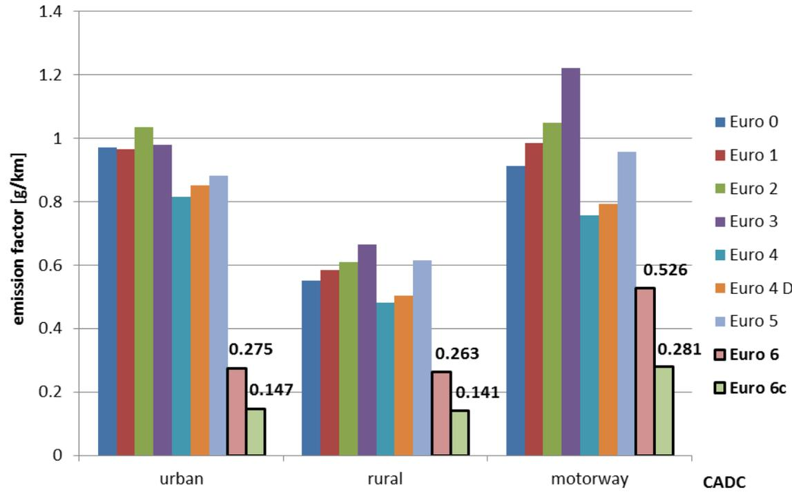
Figure 20: Emissions simulated with PHEM for diesel passenger cars in the CADC under hot start conditions
