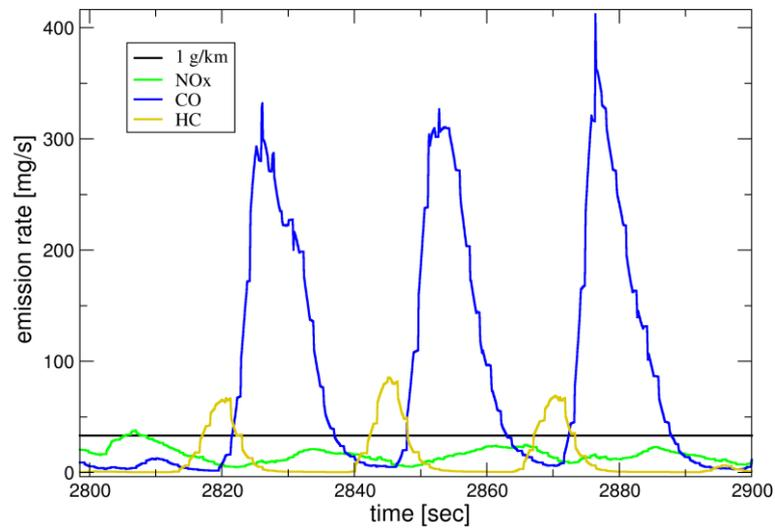
Figure 23: LNT emission control during motorway driving yielding a fast succession of regenerations with still substantial NO<sub>x</sub> emissions.
