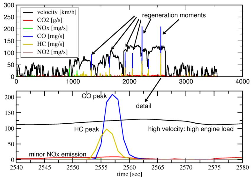
Figure 22: Typical regeneration moments at high velocities. A peak of CO and HC with limited  $\text{NO}_x$  emissions.
