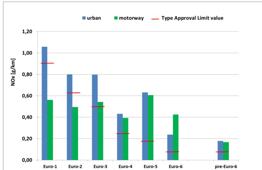
Figure 2: NOx emission factors in the city and on the highway and type approval limit values of diesel passenger cars.
