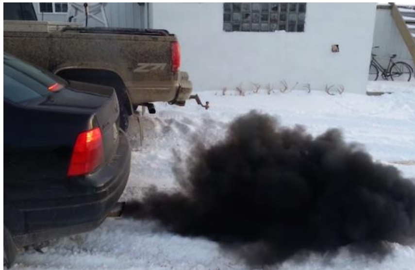
Figure 4: Example of excessive black smoke emission of a diesel engine.
