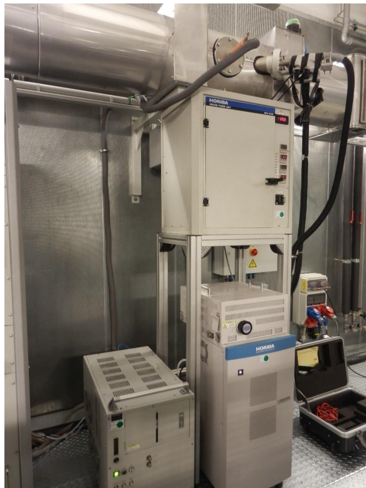
Figure 20: PM & PN type approval test equipment according to PMP-protocol.
