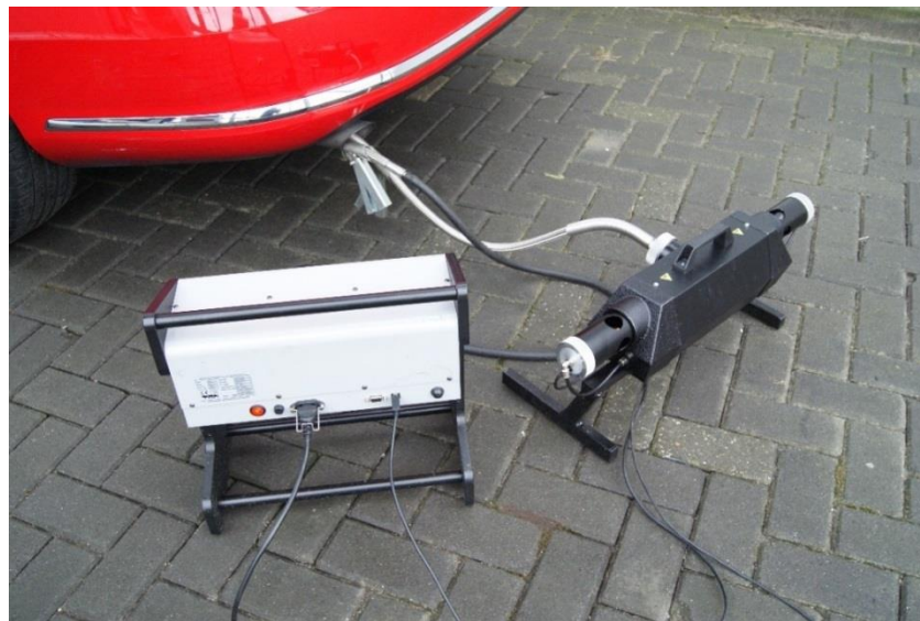
Figure 2: PTI test set up free acceleration smoke emission test with the two applied opacimeters.
