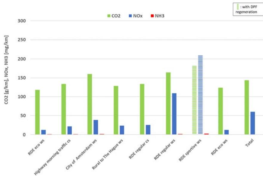
Figure A-37: Average CO<sub>2</sub>, NO<sub>x</sub>, NH<sub>3</sub> test results of the emission test programme of the Skoda Octavia
