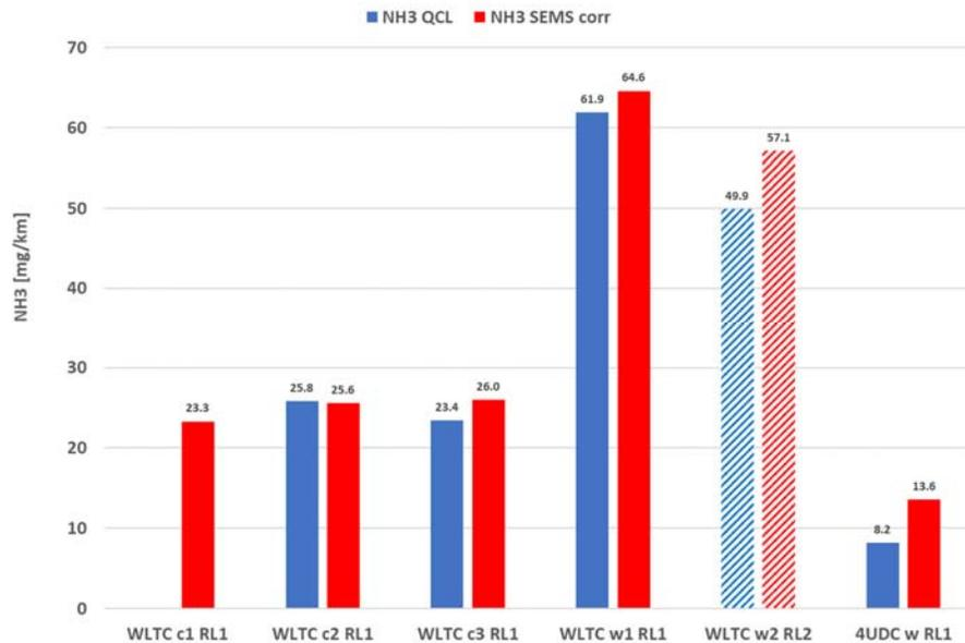
Figure A-26: WLTC and UDC NH<sub>3</sub> test results of a Peugeot Euro 6d-Temp diesel measured with QCL analyser and SEMS. In the WLTC w2 RL2 test the DPF was regenerated.
