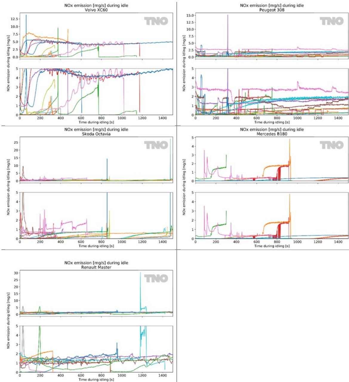
Figure 3-4: Instantaneous NO<sub>x</sub> emissions after idling has started, for all periods of extended idling. These periods are defined as when the vehicle speed is less than 5 km/h for at least 300 s. The y-axis in the top frame per vehicle is scaled automatically to show all data, while the bottom frame per vehicle shows emissions 0 – 5 mg/s.
