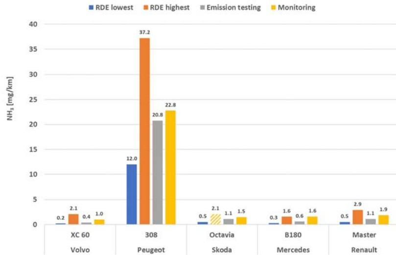
Figure A-60: NH<sub>3</sub> test results of 'RDE' tests, the emission test programme and the monitoring programme of the five tested Euro 6d-Temp diesel vehicles.
