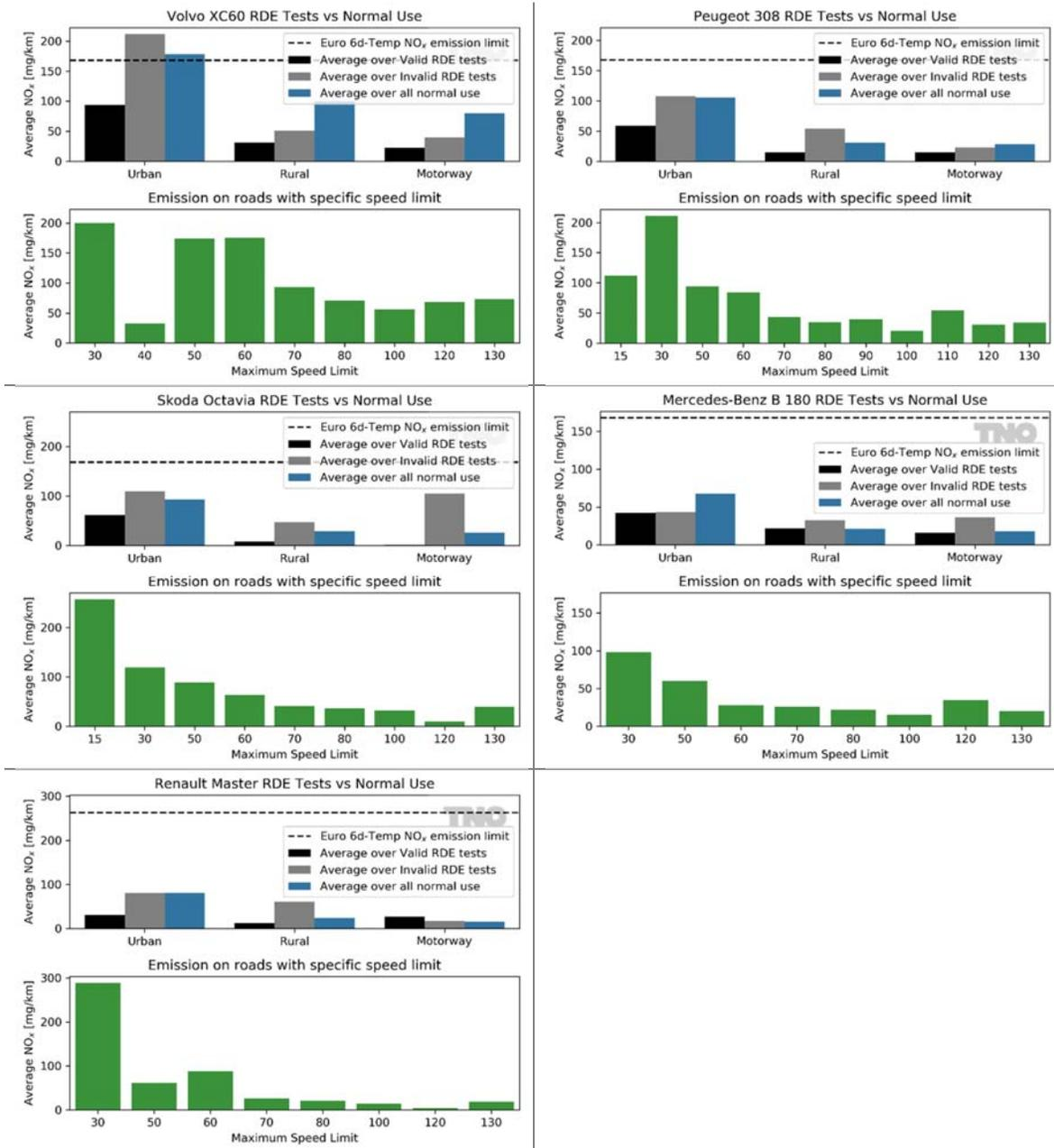
Figure 3-2: Average NO<sub>x</sub> emissions per RDE speed section for the valid and invalid RDE trips (black and grey bars) and for all normal use/monitoring (blue bars), as compared to emissions on roads with specific speed limits (green bars). Note that speed limits are only shown if the respective vehicle has spent more than 15 min on roads with that limit.
