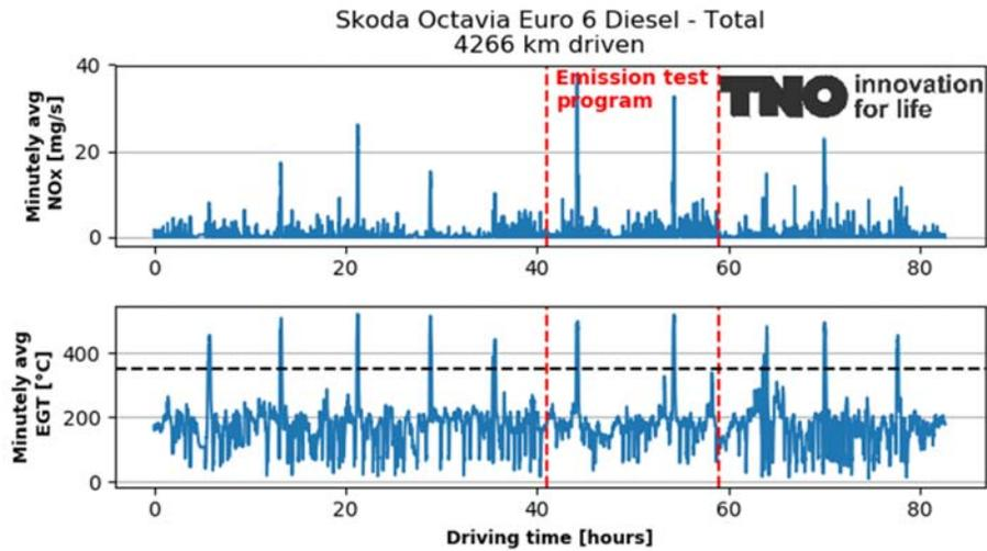
Figure A-30: NO<sub>x</sub> emission and exhaust gas temperatures over the test programme (in total 82.6 hours) of the Skoda Octavia. The red dotted lines mark the period of the emission test programme and the black dotted line marks the DPG regeneration threshold temperature.
