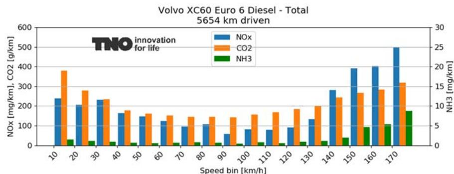
Figure A-8: Binned CO<sub>2</sub>, NO<sub>x</sub> and NH<sub>3</sub> emissions of the total test programme of the Volvo XC 60.
