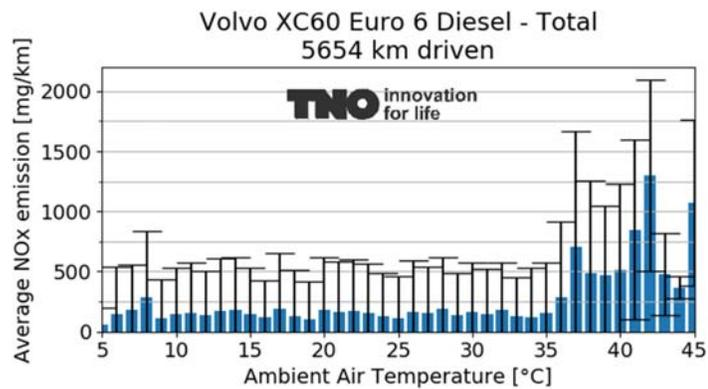
Figure A-11: Average NO<sub>x</sub> emissions per ambient air temperature bin during all driving for a Volvo XC 60. Note that the ambient air temperature is logged by the vehicle, and therefore can be affected by the state of the vehicle itself. Furthermore, this does not address the respective driving situations at these temperatures (i.e. driving behaviour can be different in summer due to a range of factors, let alone the temperature).
