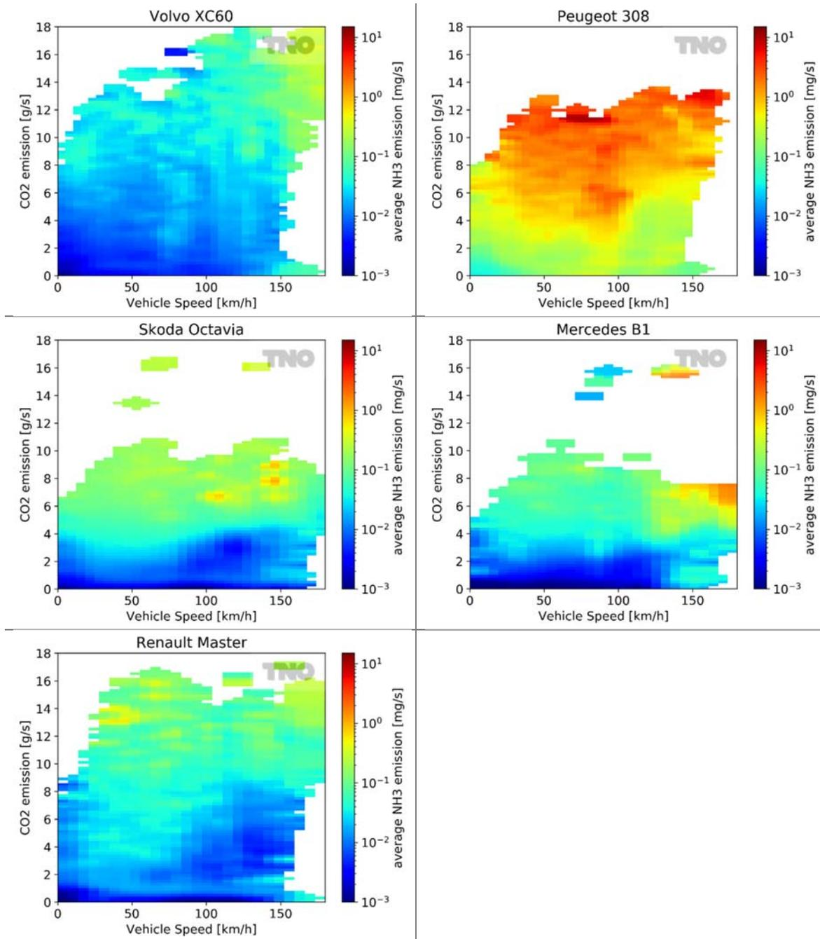
Figure 4-3: Two-dimensional emission map of average NH<sub>3</sub> emissions shown dependent on CO<sub>2</sub> emissions and vehicle speed.
