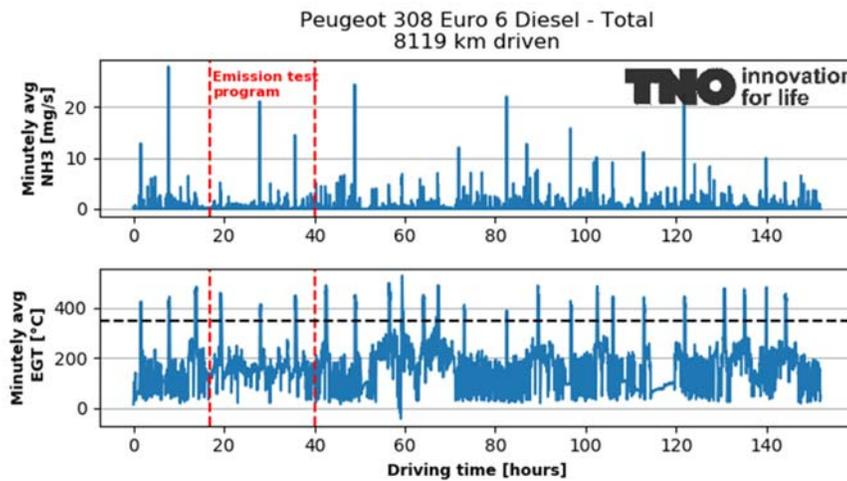
Figure A-16: NH<sub>3</sub> emission and exhaust gas temperatures over the test programme (in total 151.9 hours) of the Peugeot 308. The red dotted lines mark the period of the emission test program.
