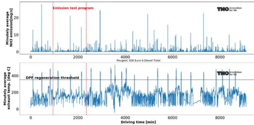
Figure A-22: Minutely average NH<sub>3</sub> emissions and exhaust gas temperature of the Peugeot 308 over all measurement data.
