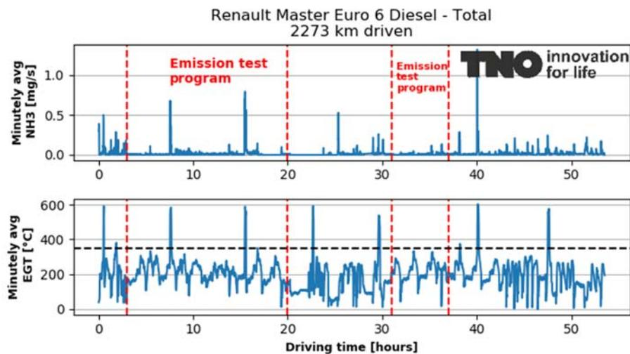
Figure A-48: NH<sub>3</sub> emission and exhaust gas temperatures over the test programme (in total 53.5 hours) of the Renault Master. The red dotted lines mark the period of the emission test program. The black dotted line marks the DPF regeneration threshold temperature.
