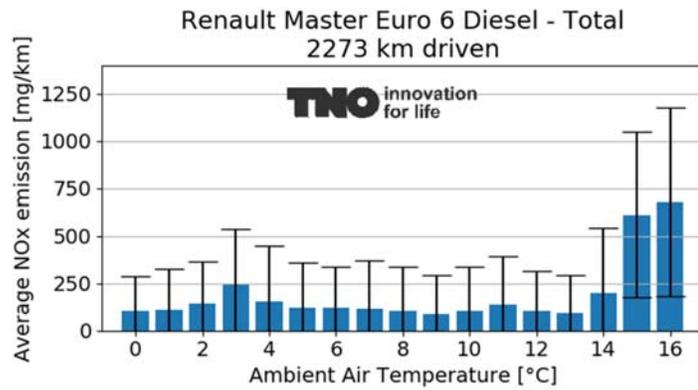
Figure A-52: Average NO<sub>x</sub> emissions per ambient air temperature bin during all driving for a Renault Master. Note that the ambient air temperature is logged by the vehicle, and therefore can be affected by the state of the vehicle itself. Furthermore, this does not address the respective driving situations at these temperatures (i.e. driving behaviour can be different in summer due to a range of factors, let alone the temperature).
