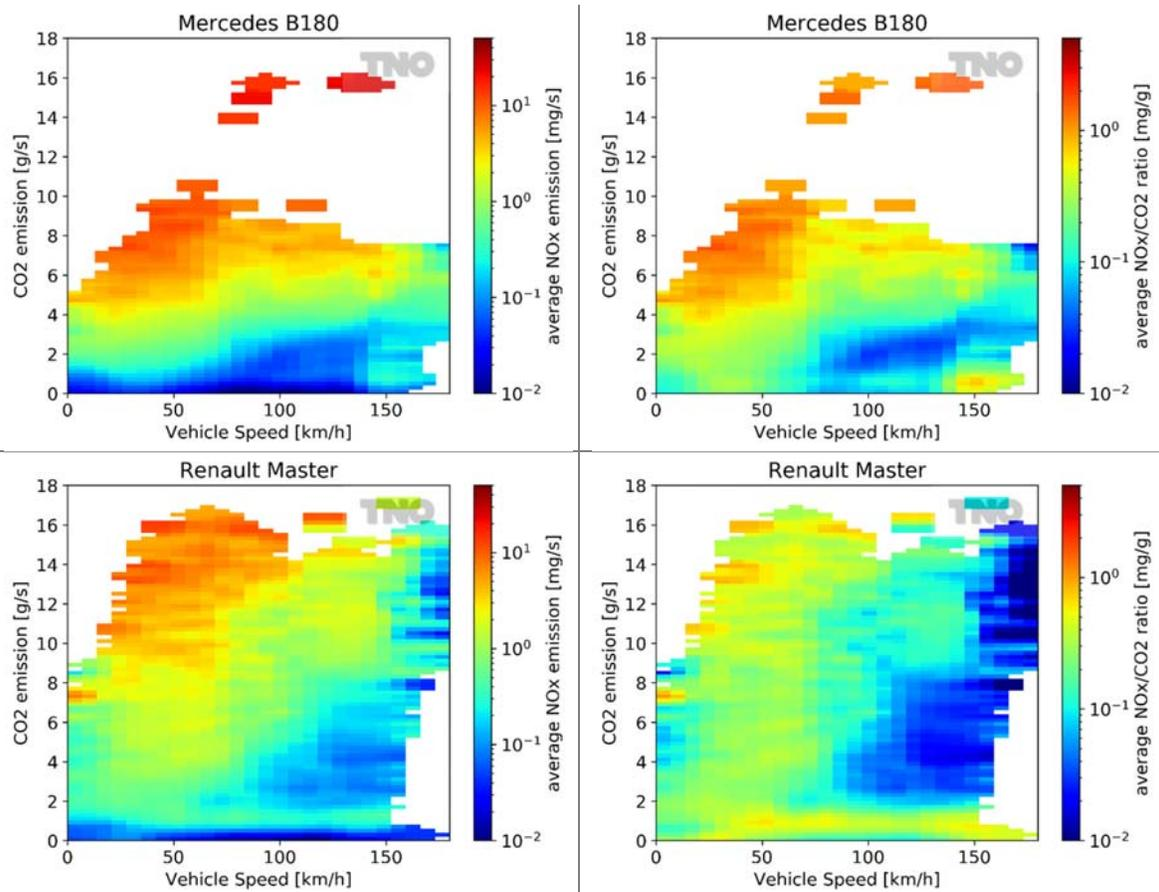
Figure 3-8: Two-dimensional emission map of average NO<sub>x</sub> emissions (left) and average NO<sub>x</sub>/CO<sub>2</sub> ratio (right), both shown dependent on CO<sub>2</sub> emissions and vehicle speed.
