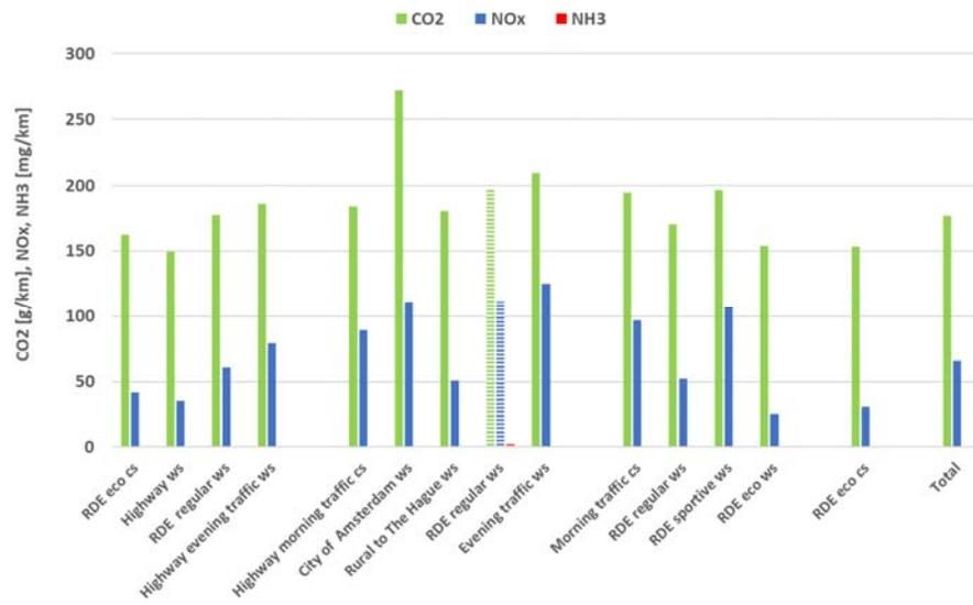
Figure A-13: Average CO<sub>2</sub>, NO<sub>x</sub> and NH<sub>3</sub> results of the emission test programme of the Volvo XC 60.
