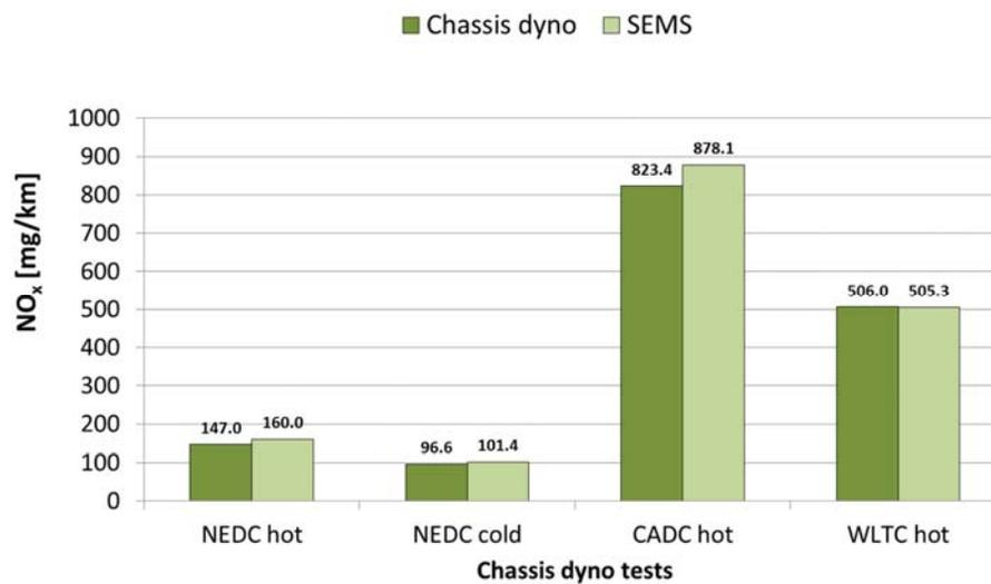
Figure A-4: NO<sub>x</sub> emissions of a Euro 6 diesel passenger car on a chassis dynamometer test: comparison of simultaneously executed measurements with the CVS/bag method of the chassis dynamometer and SEMS.
