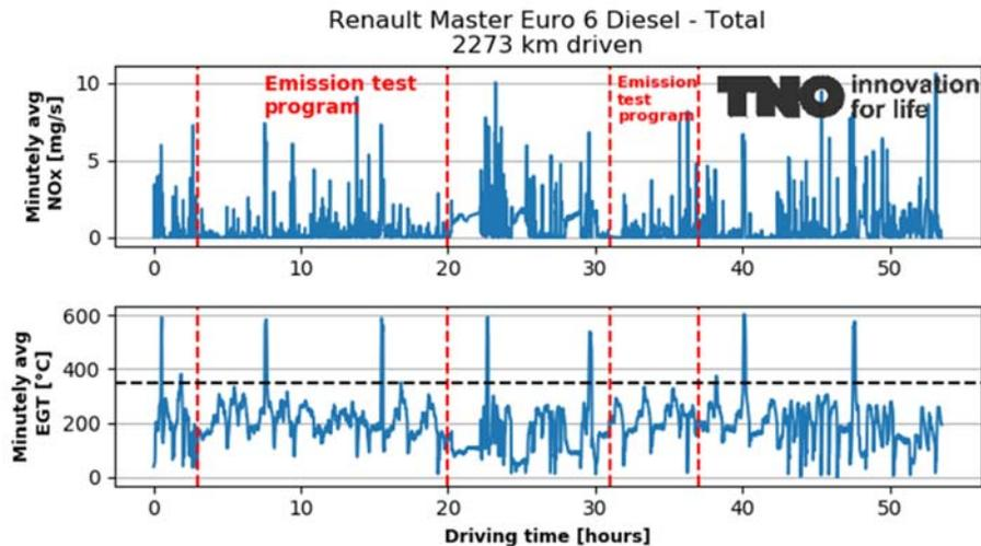
Figure A-47: NO<sub>x</sub> emission and exhaust gas temperatures over the test programme (in total 53.5 hours) of the Renault Master. The red dotted lines mark the period of the emission test program. The black dotted line marks the DPF regeneration threshold temperature.
