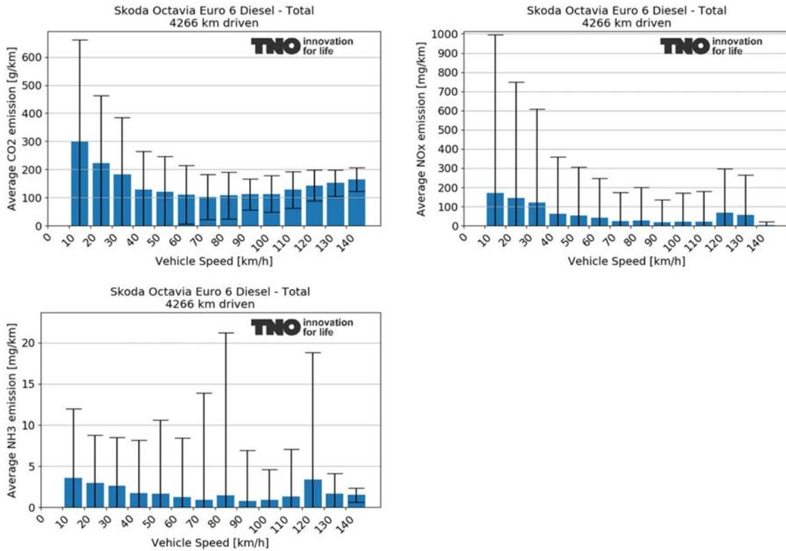
Figure A-34: Average CO<sub>2</sub>, NO<sub>x</sub> and NH<sub>3</sub> emissions dependent on vehicle speed bin during all driving for a Skoda Octavia.
