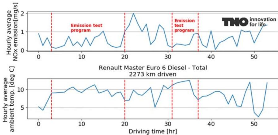
Figure A-53: NO<sub>x</sub> emission and exhaust gas temperatures over the test program of the Renault Master. The red dotted lines mark the period of the emission test program.
