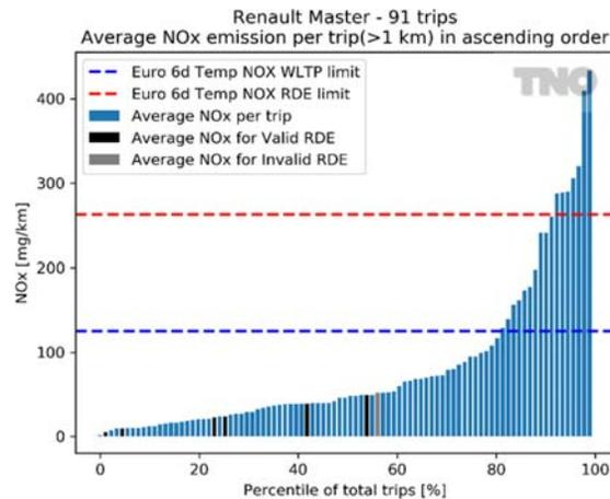
Figure 3-1: Average NO<sub>x</sub> emissions per trip for every trip driven by the five 6d-Temp vehicles, as sorted by increasing average NO<sub>x</sub>. The valid RDE trips are indicated by the black bars, while the invalid RDE trips are grey. The invalid RDE trips include, for example, the RDE trips with DPF regenerations, especially in the case of the Skoda (see also Appendix A). The WLTP and RDE limit are indicated by the blue and red dashed lines respectively.
