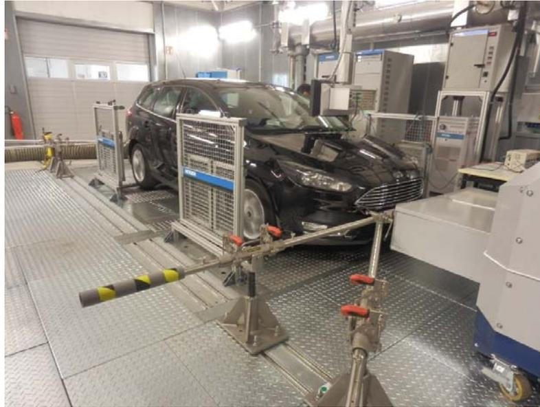
Horiba Europe GMBH carries out emission tests in its laboratory according to ISO 17025 standards and is certified for this. The following measuring equipment has been installed in the test room:
