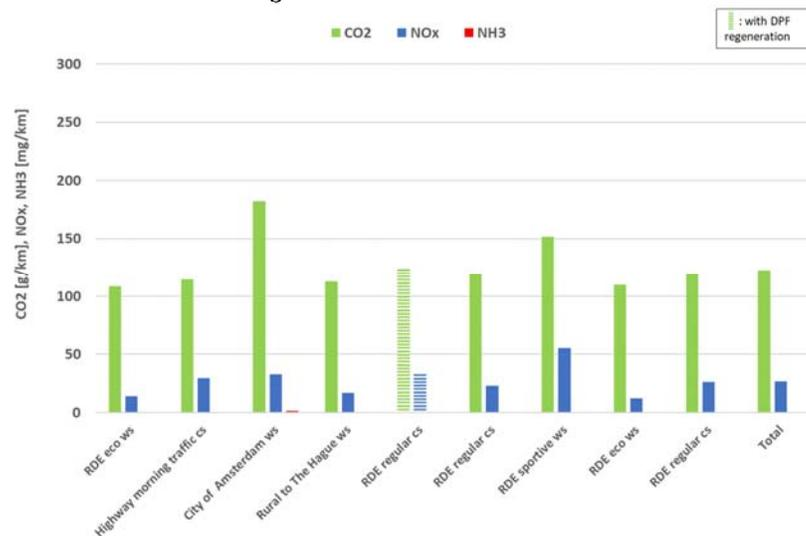
Figure A-45: Average CO<sub>2</sub>, NO<sub>x</sub>, NH<sub>3</sub> results of the emission test programme of the Mercedes B180.
