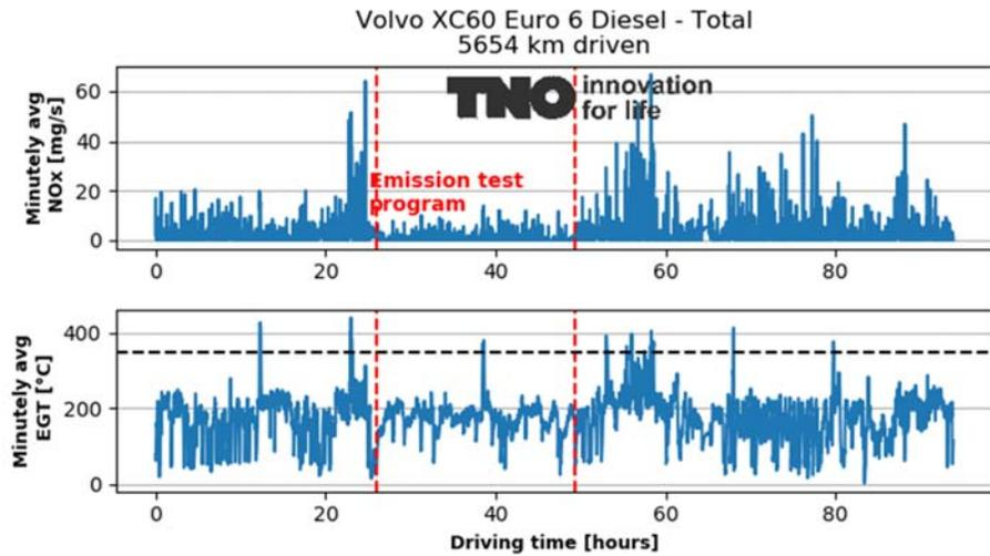
Figure A-6: NO<sub>x</sub> emission and exhaust gas temperatures over the test programme (in total 93.9 hours) of the Volvo XC 60. The red dotted lines mark the period of the emission test program.
