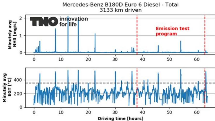
Figure A-41: NH<sub>3</sub> emission and exhaust gas temperatures over the test programme (in total 64.0 hours) of the Mercedes B180. The red dotted lines mark the period of the emission test program. The black dotted line marks the DPF regeneration threshold temperature.
