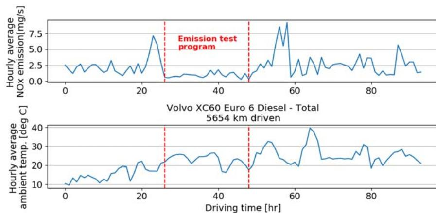
Figure A-12: NO<sub>x</sub> emission and exhaust gas temperatures over the test programme (in total 93.9 hours) of the Volvo XC 60. The red dotted lines mark the period of the emission test program.
