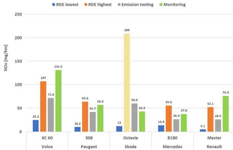
Figure A-59: NO<sub>x</sub> test results of 'RDE' tests, the emission test programme and the monitoring programme of the five tested Euro 6d-Temp diesel vehicles.
