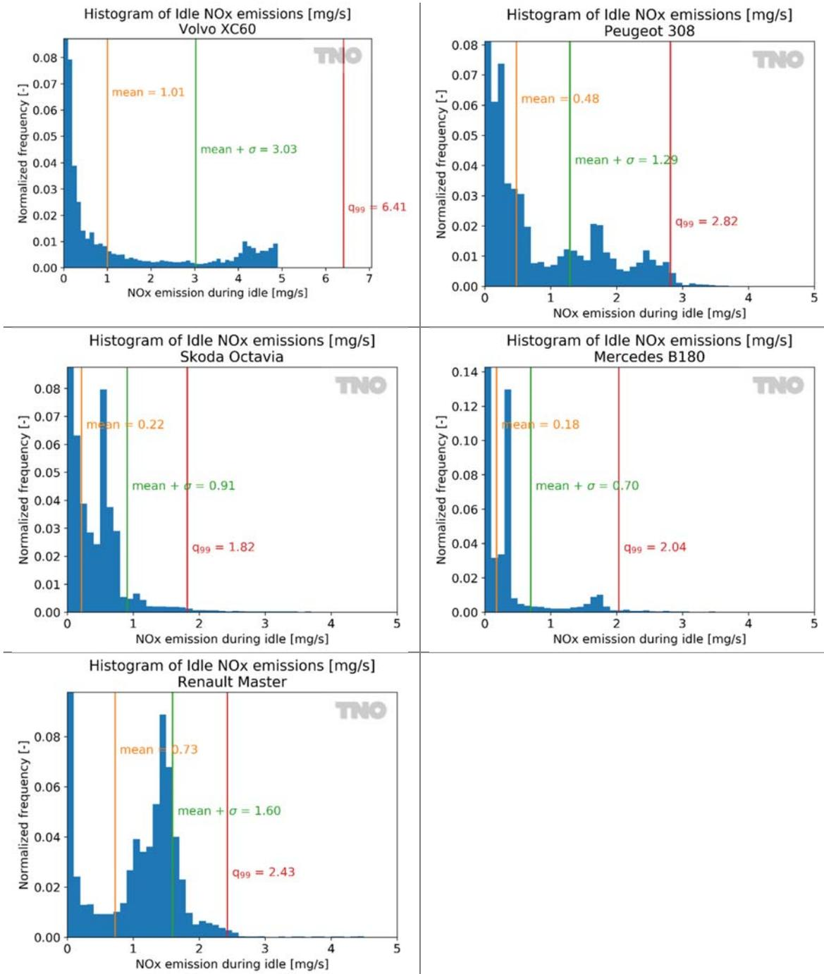
Figure 3-5: Frequency distribution of the instantaneous NO<sub>x</sub> emissions for all periods of extended idling. Idling periods are defined as when the vehicle speed is less than 5 km/h for at least 300 s. The y-axis is truncated to show the details of the emission distribution; the mean, mean + standard deviation, and 99<sup>th</sup> quantile are annotated to give a quantified indication of the distribution.
