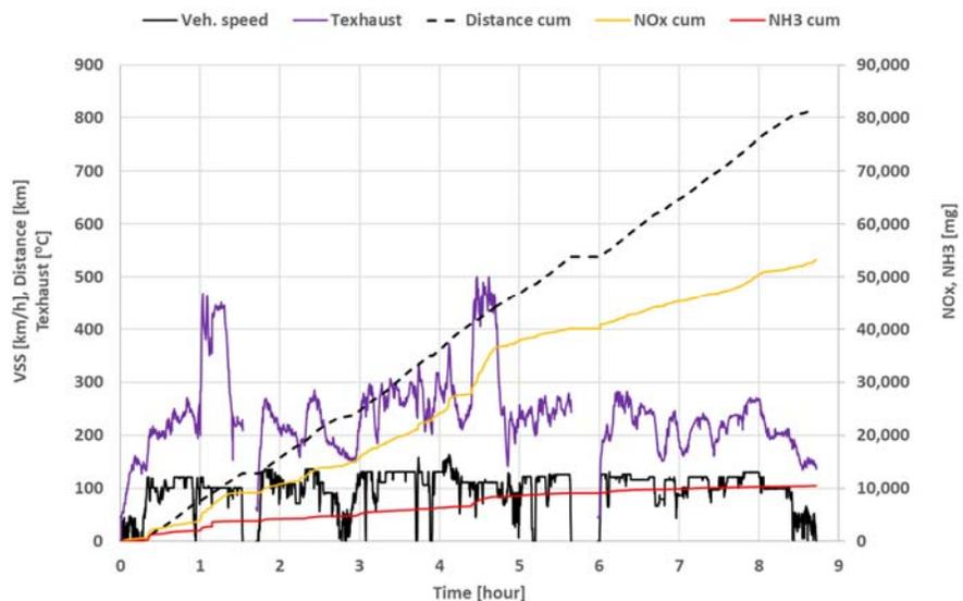
Figure A-28: Example of a long haul trip from Switzerland to The Netherlands (815 km, average vehicle speed 99.4 km/h). The average emissions were CO<sub>2</sub> 133 g/km, NO<sub>x</sub> 65 mg/k0m and NH<sub>3</sub> 13 mg/km. The DPF was regenerated two times during 20 minutes, the interval was 333 km).
