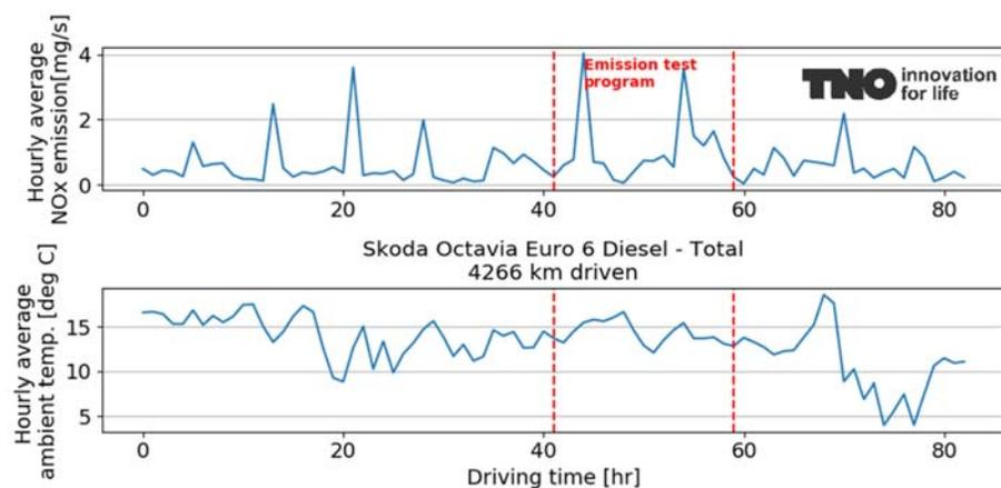
Figure A-36: NO<sub>x</sub> emission and exhaust gas temperatures over the test program of the Skoda Octavia. The red dotted lines mark the period of the emission test program.
