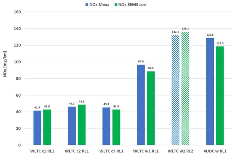
Figure A-25: WLTC and UDC NO<sub>x</sub> test results of a Peugeot Euro 6d-Temp diesel measured with CVS and SEMS. In the WLTC w2 RL2 test the DPF was regenerated.
