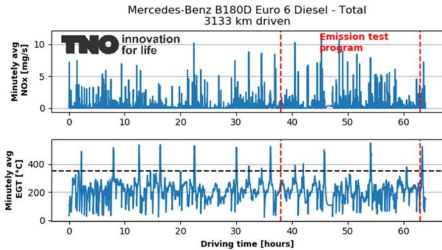
Figure A-40: NO<sub>x</sub> emission and exhaust gas temperatures over the test programme (in total 64.0 hours) of the Mercedes B180. The red dotted lines mark the period of the emission test program. The black dotted line marks the DPF regeneration threshold temperature.
