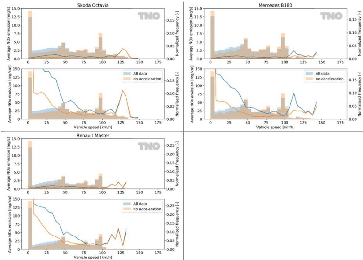
Figure 3-7: Average NO<sub>x</sub> (lines) and frequency distribution (bars) per speed bin for all data and data excluding acceleration (acceleration less than 0.5 m/s<sup>2</sup>, equivalent to 1.8 km/h per second).
