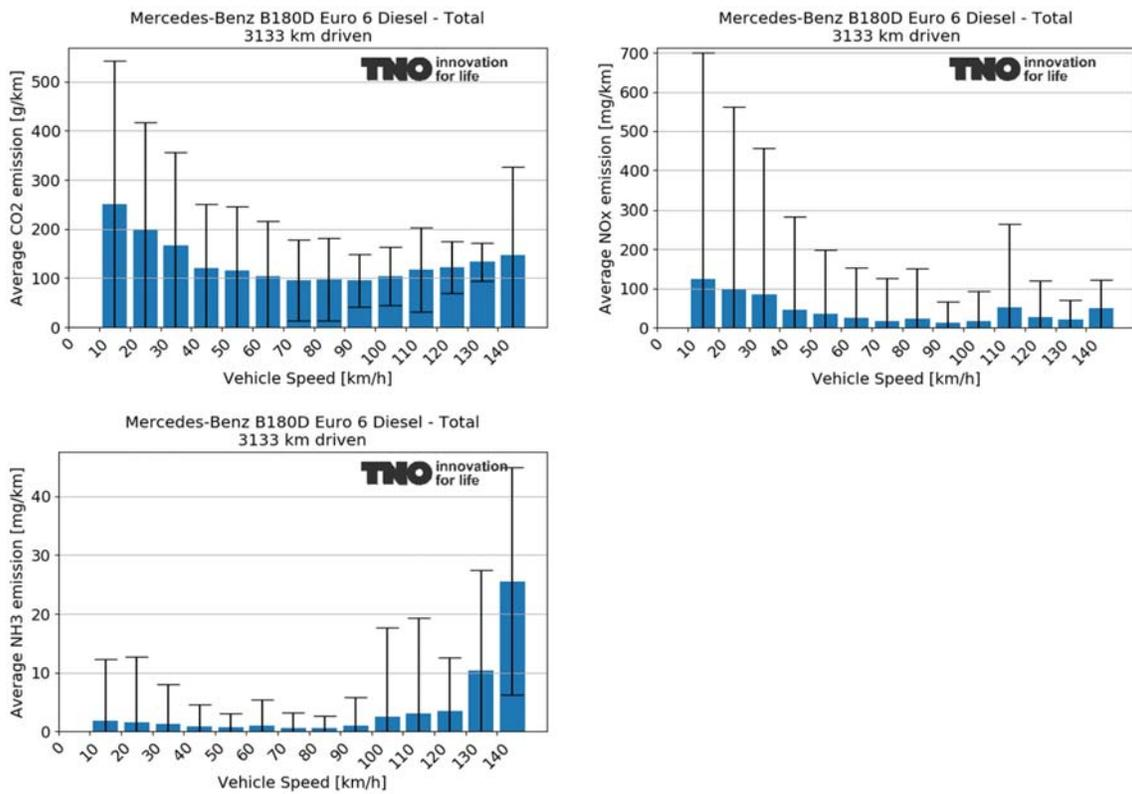
Figure A-44: Average CO<sub>2</sub>, NO<sub>x</sub> and NH<sub>3</sub> emissions dependent on vehicle speed bin during all driving for a Mercedes B180
