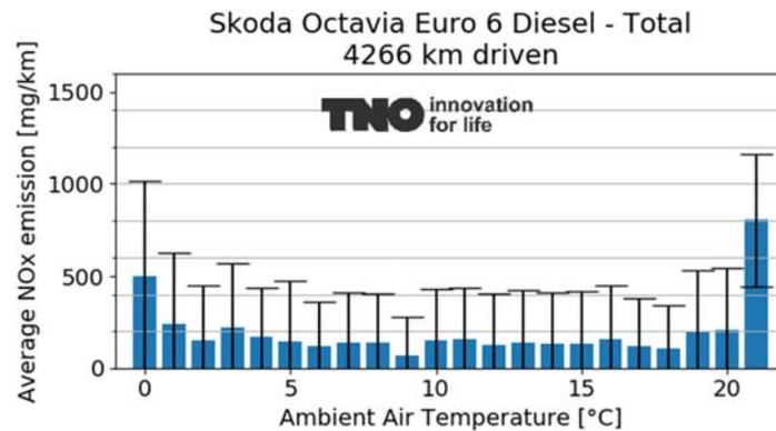
Figure A-35: Average NO<sub>x</sub> emissions per ambient air temperature bin during all driving for a Skoda Octavia. Note that the ambient air temperature is logged by the vehicle, and therefore can be affected by the state of the vehicle itself. Furthermore, this does not address the respective driving situations at these temperatures (i.e. driving behaviour can be different in summer due to a range of factors, let alone the temperature).
