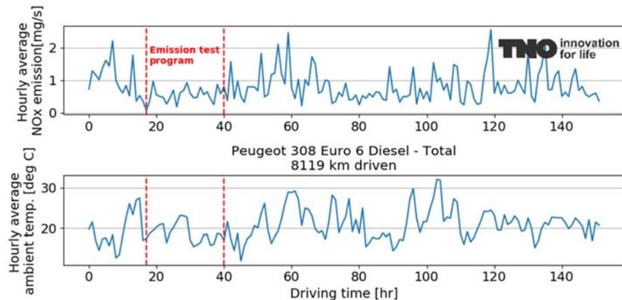
Figure A-21: NO<sub>x</sub> emission and exhaust gas temperatures over the test programme (in total 151.9 hours) of the Peugeot 308. The red dotted lines mark the period of the emission test program.
