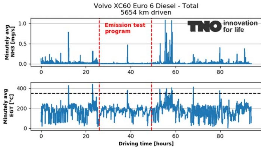
Figure A-7: NH<sub>3</sub> emission and exhaust gas temperatures over the test programme (in total 93.9 hours) of the Volvo XC 60. The red dotted lines mark the period of the emission test program.
