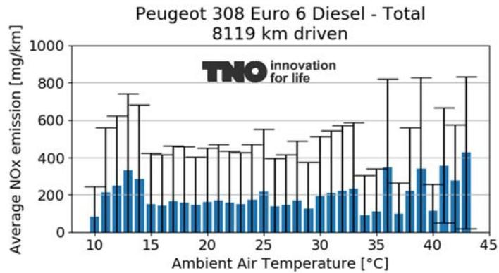
Figure A-20: Average NO<sub>x</sub> emissions per ambient air temperature bin during all driving for a Peugeot 308. Note that the ambient air temperature is logged by the vehicle, and therefore can be affected by the state of the vehicle itself. Furthermore, this does not address the respective driving situations at these temperatures (i.e. driving behaviour can be different in summer due to a range of factors, let alone the temperature).
