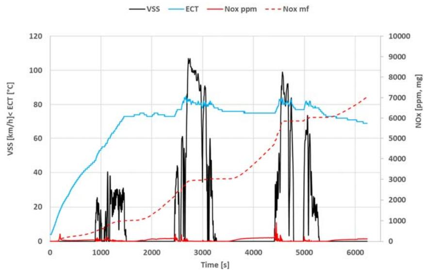
Figure A-56: Trip of 105 minutes with cold start and idling periods of a Euro 6d-Temp Renault Master with ambient temperatures of 1 – 7 °C. Average speed is 14.4 km/h, CO<sub>2</sub> 352 g/km, NO<sub>x</sub> 287 mg/km.
