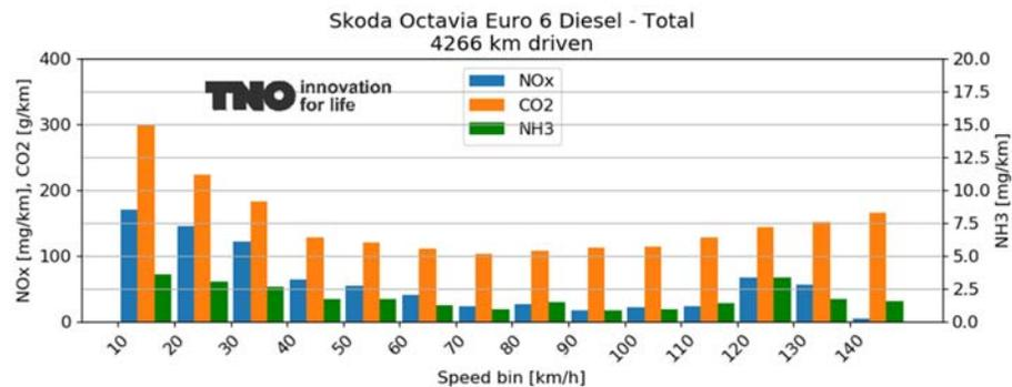
Figure A-32: Binned CO<sub>2</sub>, NO<sub>x</sub> and NH<sub>3</sub> emissions of the total test programme of the Skoda Octavia.
