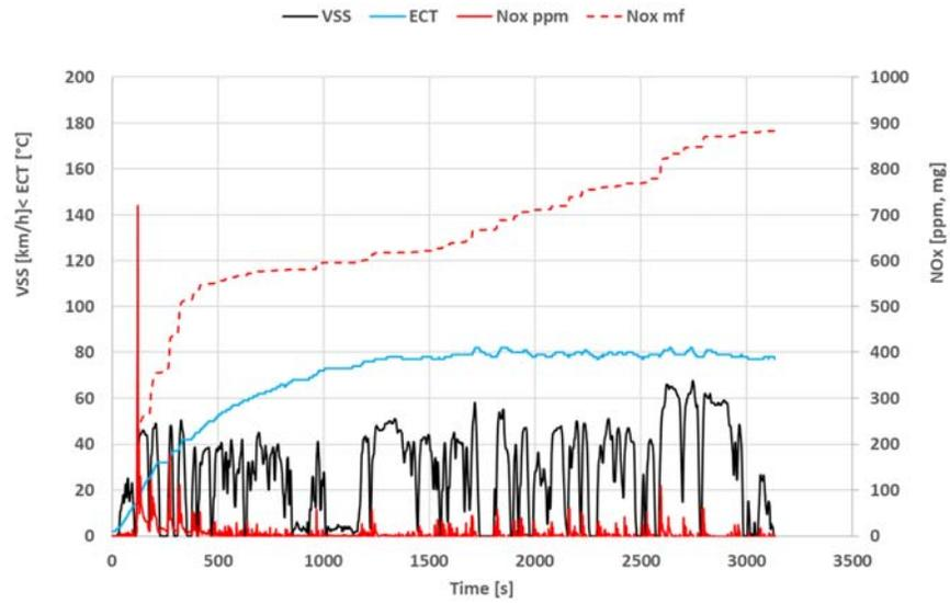
Figure A-55: Urban trip of 51 minutes with cold start of a Euro 6d-Temp Renault Master with ambient temperatures of 0 – 3 °C. Average speed is 27.9 km/h, CO<sub>2</sub> 256 g/km, NO<sub>x</sub> 37 mg/km.
