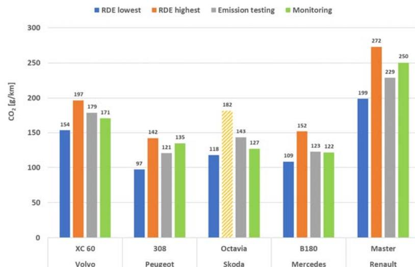
Figure A-58: CO<sub>2</sub> test results of 'RDE' tests, the emission test programme and the monitoring programme of the five tested Euro 6d-Temp diesel vehicles.
