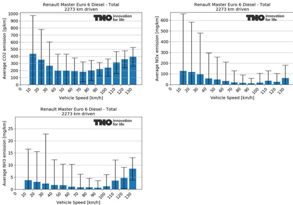
Figure A-51: Average CO<sub>2</sub>, NO<sub>x</sub> and NH<sub>3</sub> emissions dependent on vehicle speed bin during all driving for a Renault Master
