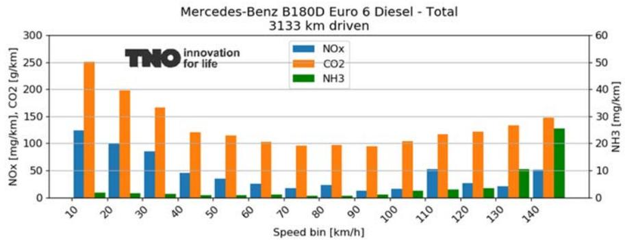
Figure A-42: Binned CO<sub>2</sub>, NO<sub>x</sub> and NH<sub>3</sub> emissions of the total test programme of the Mercedes B180.
