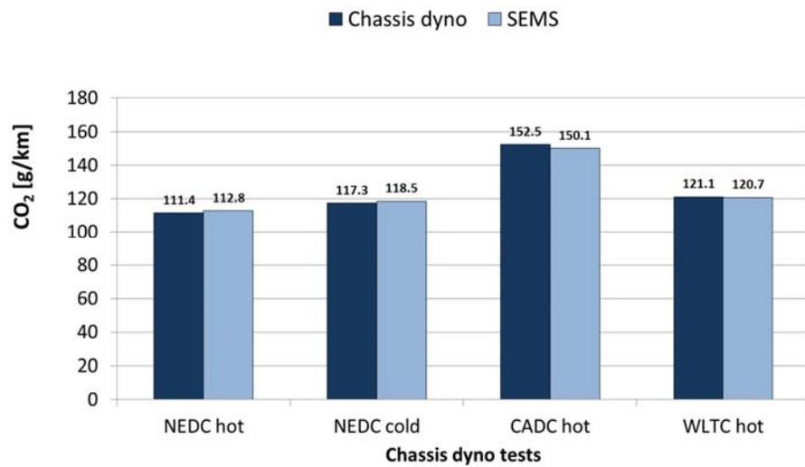
Figure A-3: CO<sub>2</sub> emissions of a Euro 6 diesel passenger car on a chassis dynamometer test: comparison of simultaneously executed measurements with the CVS/bag method of the chassis dynamometer and SEMS.
