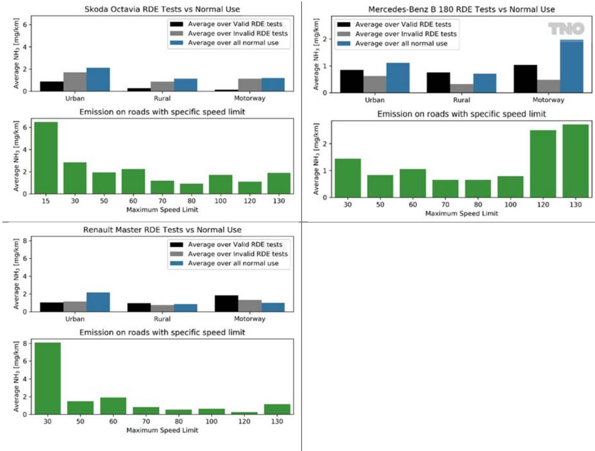
Figure 4-1: Average NH<sub>3</sub> emissions per RDE speed section for the 'RDE' trips (blue bars) and for all normal use/monitoring (orange bars), as compared to emissions on roads with specific speed limits (green bars). Note that speed limits are only shown if the respective vehicle has spent more than 15 min on roads with that limit.
