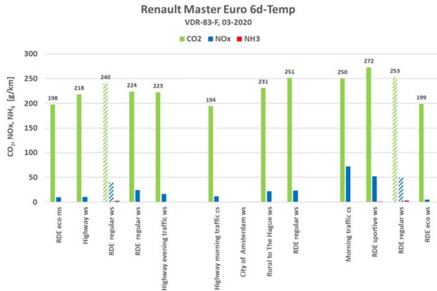
Figure A-54: Average CO<sub>2</sub>, NO<sub>x</sub>, NH<sub>3</sub> results of the emission test programme of the Renault Master.
