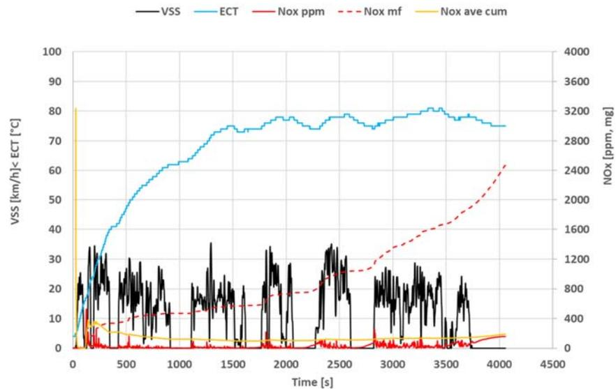
Figure A-57: Delivery trip of 66 minutes with cold start of a Euro 6d-Temp Renault Master with ambient temperatures of 0 – 3 °C. Average speed is 11.5 km/h, CO<sub>2</sub> 367 g/km, NO<sub>x</sub> 198 mg/km.
