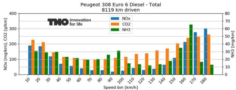
Figure A-18: Binned CO<sub>2</sub>, NO<sub>x</sub> and NH<sub>3</sub> emissions of the total test programme of the Peugeot 308.
