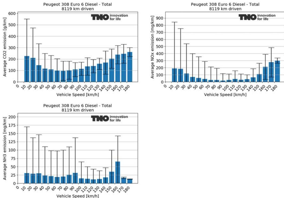
Figure A-17: Average CO<sub>2</sub>, NO<sub>x</sub> and NH<sub>3</sub> emissions dependent on vehicle speed bin during all driving for a Peugeot 308.
