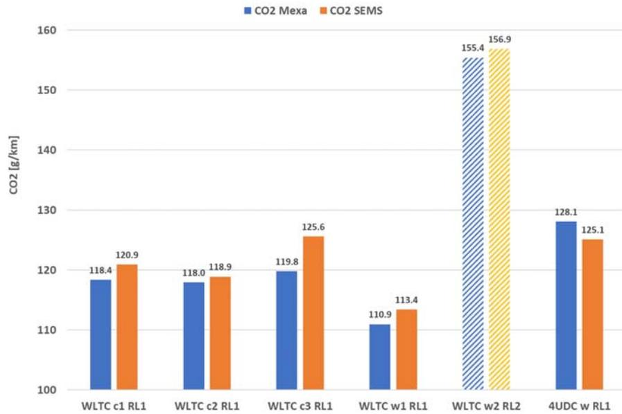
Figure A-24: WLTC and UDC CO<sub>2</sub> test results of a Peugeot Euro 6d-Temp diesel measured with CVS and SEMS. In the WLTC w2 RL2 test the DPF was regenerated.
