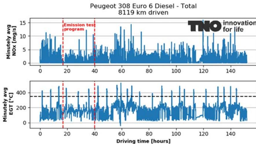
Figure A-15: NO<sub>x</sub> emission and exhaust gas temperatures over the test programme (in total 151.9 hours) of the Peugeot 308. The red dotted lines mark the period of the emission test program.
