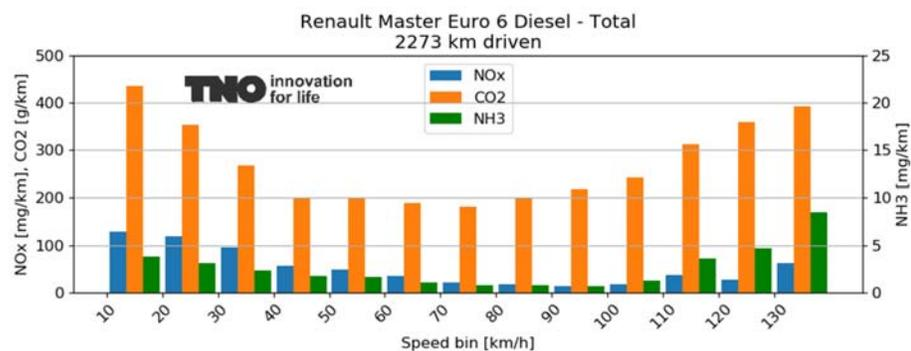
Figure A-49: Binned CO<sub>2</sub>, NO<sub>x</sub> and NH<sub>3</sub> emissions of the total test programme of the Renault Master.
