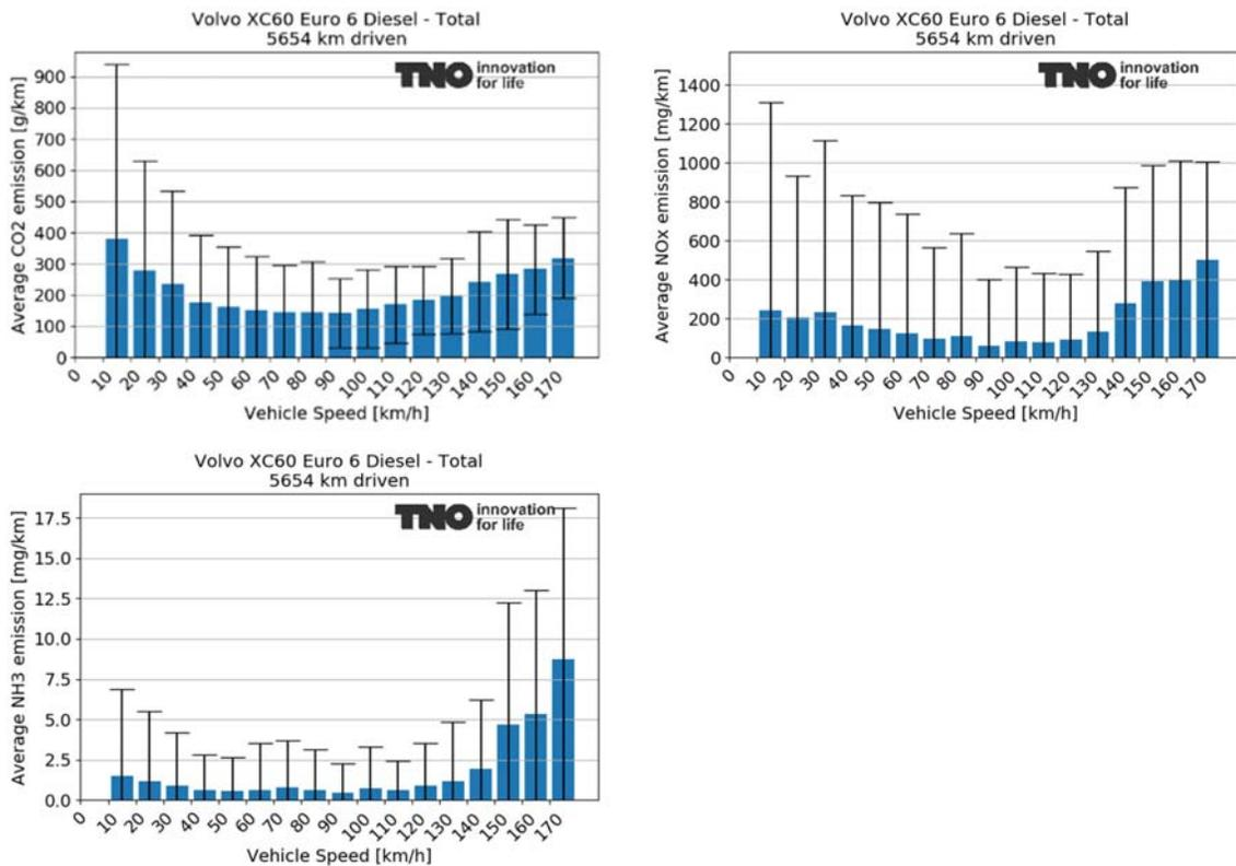
Figure A-10: Average CO<sub>2</sub>, NO<sub>x</sub> and NH<sub>3</sub> emissions dependent on vehicle speed bin during all driving for a Volvo XC 60.
