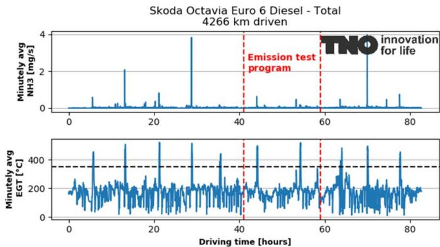
Figure A-31: NH<sub>3</sub> emission and exhaust gas temperatures over the test programme (in total 82.6 hours) of the Skoda Octavia. The red dotted lines mark the period of the emission test programme and the black dotted line marks the DPG regeneration threshold temperature.
