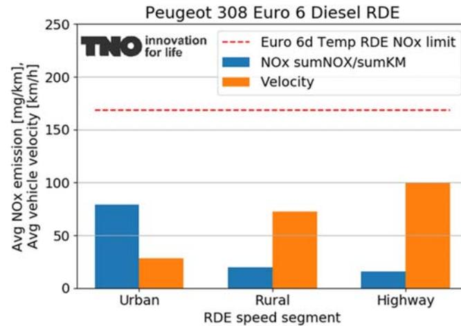
Figure A-19: Average velocities and average NO<sub>x</sub> emissions in the urban, rural and highway parts of the 'RDE' test of a Peugeot 308.
