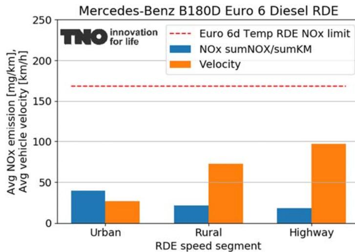
Figure A-43: Average velocities and average NO<sub>x</sub> emissions in the urban, rural and highway parts of the 'RDE' tests of a Mercedes B180.
