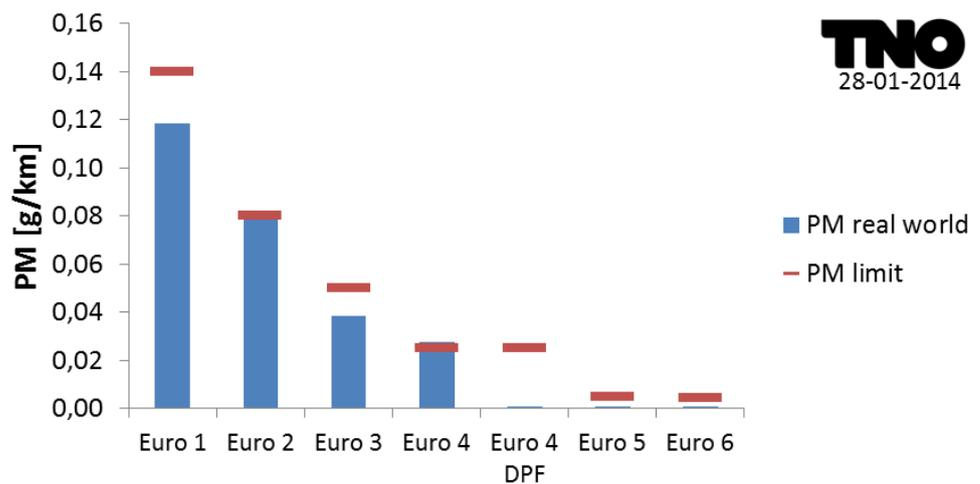
Figure 4: PM emission factors and type approval limit values of diesel passenger cars
