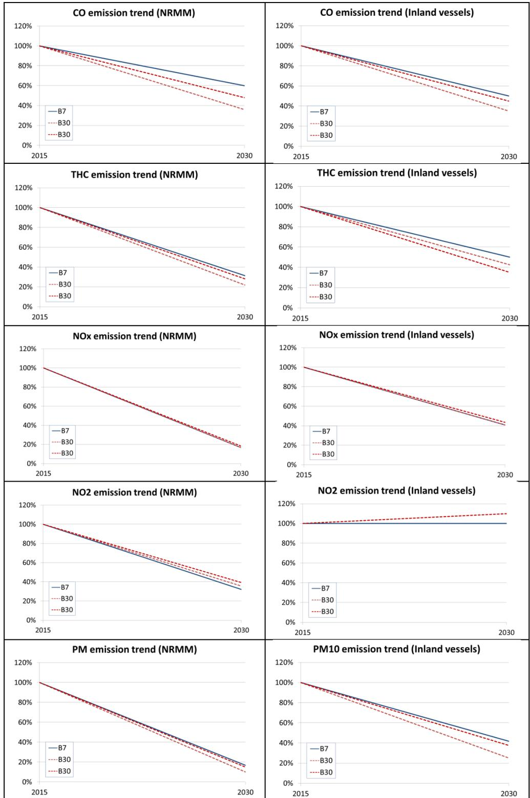
Figure 12: Emissions trends 2015-2030 –Inland vessels and Non-road mobile machinery (NRMM)
