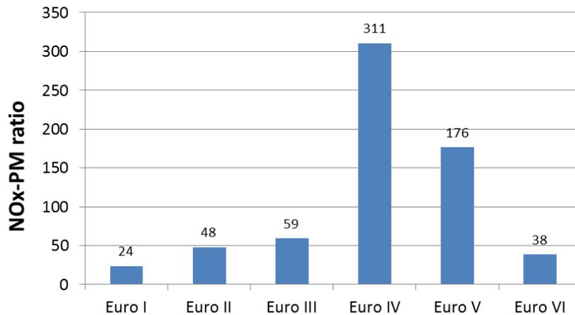
Figure 9: NOx-PM ratios of Heavy Duty vehicles
