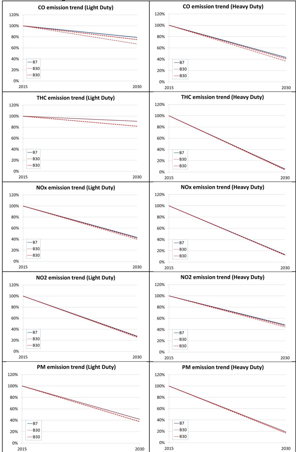
Figure 11: Predicted emissions trends 2015-2030 – Light Duty and Heavy Duty vehicles and the effects of increased biodiesel blends.
