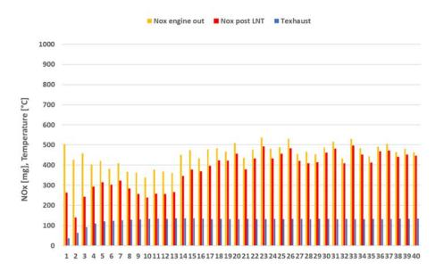
Figure 5-9:  $NO_x$  emissions per ECE cycle with engine calibration 2 in a 10\*UDC test with a cold start, start-stop active, performed on 8-11-2018. The test was started in a conditioning room of 26 °C and was conducted on the test track of the RDW at an ambient temperature of 13 °C. Preconditioning 3\*EUDC with a warm start, conducted on 7-11-2018, with 2 LNT regenerations in the second and third EUDC cycles.
