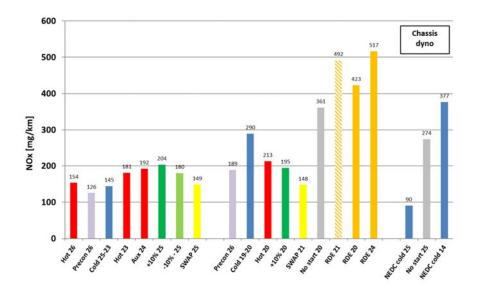
Figure 1-1:  $NO_x$  test results from initial exploratory measurements in a RDW study from 2017 on a Suzuki Vitara Euro 6b diesel. The diesel particulate filter has been regenerated in the RDE test using the shaded bar.
