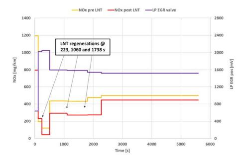
Figure 5-19: Average NO<sub>x</sub> emissions, measured at a constant speed of 110 km/h with SEMS and a vehicle with a cold engine start and engine calibration 2, performed on 18-07-2019. The test was conducted on the test track at an ambient temperature of 26°C. Preconditioning test 20 minutes @ 130 km/h.
