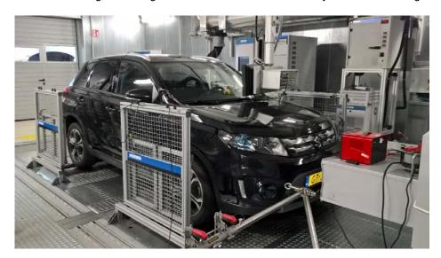
Figure 2-1: A Suzuki Vitara on the chassis dynamometer.
