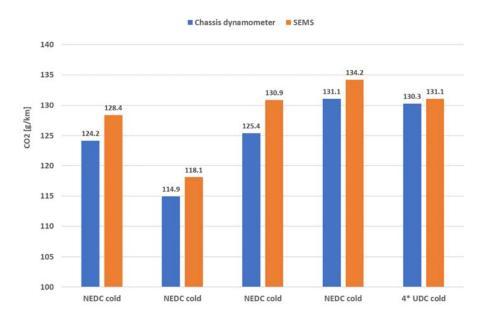
Figure 4-28: CO<sub>2</sub> emissions with engine calibration 1 from different chassis dynamometer tests measured with the chassis dynamometer equipment and with the SEMS.
