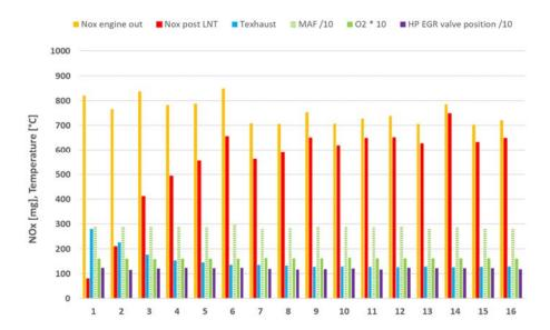
Figure 4-20: NO<sub>x</sub> emissions per ECE cycle with engine calibration 1 in a 4\*UDC test with a warm start, performed on 24-04-2018. The test was started and driven on the test track of the RDW at an ambient temperature of 14 °C. Preconditioning 120 km/h with a warm start with various LNT regenerations.
