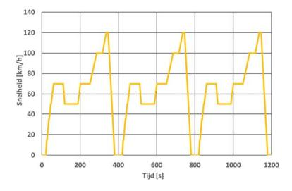
Figure 2-4: Test Cycle (3\*EUDC) for preconditioning of the Suzuki Vitara.
