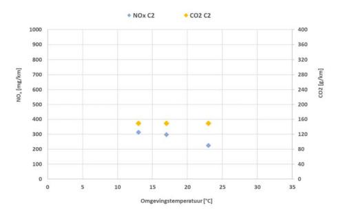
Figure 5-3: Corrected NO<sub>x</sub> and CO<sub>2</sub> emissions of NEDC tests with a cold start, measured on the test track with engine calibration 2 at different ambient temperatures
