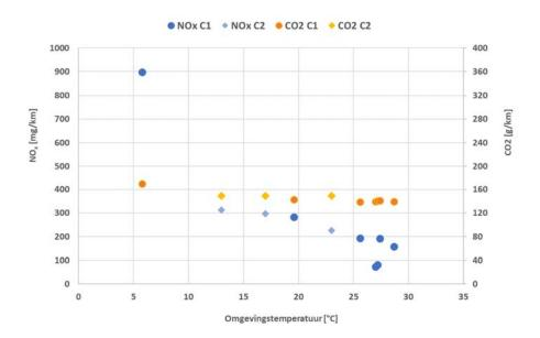
Figure 6-1: Corrected NO<sub>x</sub> and CO<sub>2</sub> emissions of NEDC tests with a cold start, measured on the test track with engine calibration 1 and 2 at different ambient temperatures.
