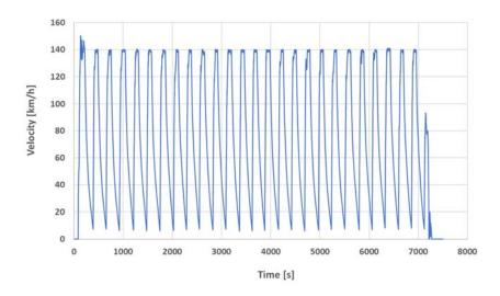
Figure 5-1: Road load testing of the Suzuki Vitara on the test track in Lelystad with six different starting points on the test track
