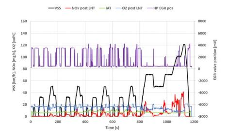
Figure 4-9: NEDC test of 29-03-2018, with engine calibration 1 and a cold start, conducted on the test track at an ambient temperature of 6 °C. The NO<sub>x</sub> emission is 533 mg/km. A preconditioning test with 1 LNT regeneration (8 seconds) was conducted prior to this NEDC test on 29-03-2018.
