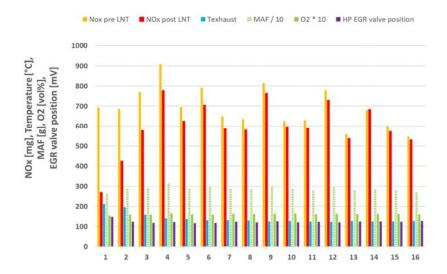
Figure 4-18: NO<sub>x</sub> emissions per ECE cycle with engine calibration 1 in a 4\*UDC test with a warm start, performed on 16-04-2018. The test was started and driven on the test track of the RDW at an ambient temperature of 18 °C. Preconditioning 10 minutes @ 120 km/h with a warm start without LNT regenerations.
