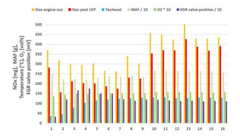
Figure 4-16: NO<sub>x</sub> emissions per ECE cycle with engine calibration 1 in a 4\*UDC test with a cold start, performed on 25-05-2018. The test was started in a conditioning room of 26°C and was conducted on the test track of the RDW at an ambient temperature of 20°C. Preconditioning 3\*EUDC with a warm start, conducted on 22-05-2018, with three LNT regenerations of 12, 12 and 8 seconds.
