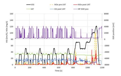
Figure 4-10: NEDC test of 14-05-2018, with engine calibration 1 and a warm start, conducted on the test track at an ambient temperature of 26-28 °C. The NO<sub>x</sub> emission is 266 mg/km. A LNT regeneration of 14 seconds takes place at approximately 90 km/h. A preconditioning test with 1 LNT regeneration (7 seconds) was conducted prior to this NEDC test on 14-05-2018.
