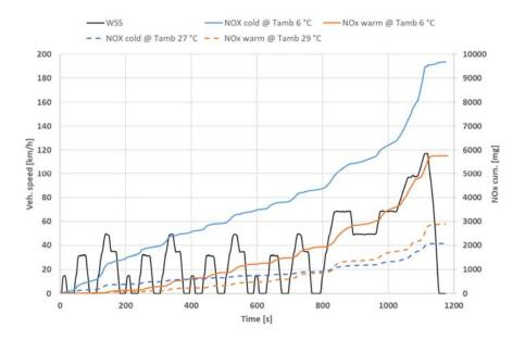
Figure 4-11: Cumulative NO<sub>x</sub> emissions from engine calibration 1 in NEDC tests with a cold and warm starts at different ambient temperatures.
