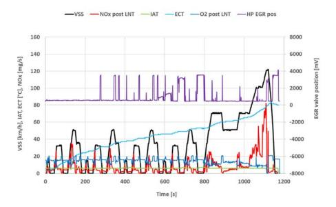
Figure 4-7: NEDC test of 29-03-2018, with engine calibration 1 and a cold start, conducted on the test track at an ambient temperature of 6 °C. The NO<sub>x</sub> emission is 897 mg/km.
