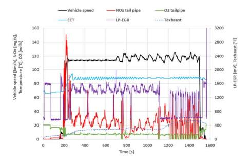
Figure 5-14:  $NO_x$  and  $O_2$  emissions measured at a constant speed of 115 - 120 km/h (warm start) with SEMS with engine calibration 2, performed on 16-04-2019. The test was conducted on the test track at an ambient temperature of 21 °C. The position signal of the low-pressure EGR valve is also shown. From t = 1100 - 1550 s the diesel particulate filter is regenerated.
