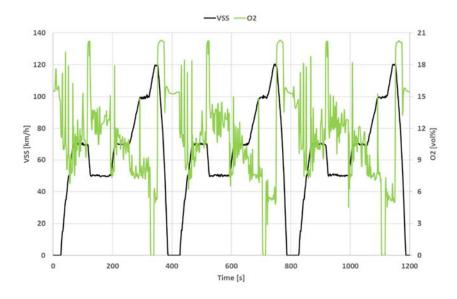
Figure 5-4: 3\*EUDC test with engine calibration 2 and warm start, conducted on 24-10-2018 on the test track, at an ambient temperature of 17 °C. The LNT is regenerated three times for 11-13 seconds.
