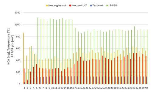
Figure 5-11: NO<sub>x</sub> emissions per ECE cycle with engine calibration 2 in a 10\*UDC test with a cold start, start-stop active, performed on 07-05-2019. The test was started in a conditioning room of 25 °C and was conducted on the test track of the RDW at an ambient temperature of 13 °C. Preconditioning 3\*EUDC with a warm start, conducted on 02-05-2018 with 3 LNT regenerations.
