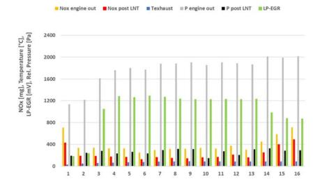
Figure 5-10: NO<sub>x</sub> emissions per ECE cycle with engine calibration 2 in a 10\*UDC test with a cold start, start-stop active, performed on 23-04-2019. The test was started in a conditioning room of 25 °C and was conducted on the test track of the RDW at an ambient temperature of 23 °C. Preconditioning 3\*EUDC with a warm start, conducted on 18-04-2018, with 2 LNT regenerations in the second and third EUDC cycles.
