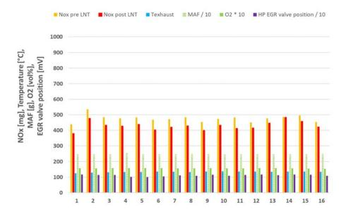
Figure 4-19:  $NO_x$  emissions per ECE cycle with engine calibration 1 in a 4\*UDC test with a warm start, performed on 19-04-2018. The test was started and driven on the test track of the RDW at an ambient temperature of 30-32 °C. Preconditioning 4\*UDC with a cold start without LNT regenerations.
