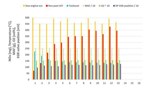
Figure 4-21:  $NO_x$  emissions per ECE cycle with engine calibration 1 in a 4\*UDC test with a warm start, performed on 22-05-2018. The test was started and driven on the test track of the RDW at an ambient temperature of 25 °C. Preconditioning 3\*EUDC with warm start, with 3 LNT regenerations.
