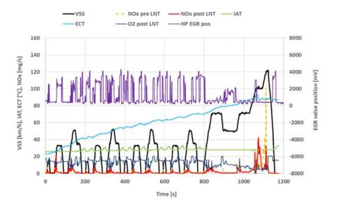
Figure 4-8: NEDC test of 14-05-2018, with engine calibration 1 and a cold start, conducted on the test track at an ambient temperature of 27-28 °C. The NO<sub>x</sub> emission is 191 mg/km. A LNT regeneration of 8 seconds takes place at 95 km/h. A preconditioning test with 3 LNT regenerations (12-12-1 seconds) was conducted prior to this NEDC test on 11-03-2018.
