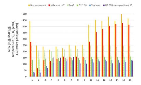
Figure 4-14: NO<sub>x</sub> emissions per ECE cycle with engine calibration 1 in a 4\*UDC test with a cold start, performed on 19-04-2018. The test was started in a conditioning room of 26°C and was conducted on the test track of the RDW at an ambient temperature of 30-32°C. Preconditioning 3\*EUDC with a warm start, conducted on 18-04-2018, with three LNT regenerations of 12, 10 and 7 seconds.
