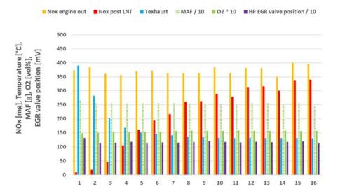
Figure 4-22: NO<sub>x</sub> emissions per ECE cycle with engine calibration 1 in a 4\*UDC test with a warm start, performed on 25-05-2018. The test was started and driven on the test track of the RDW at an ambient temperature of 22 °C. Preconditioning 120 km/h with warm start, with 5 LNT regenerations.
