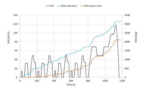
Figure 5-6: Cumulative  $NO_x$  emissions from NEDC tests with a cold and warm start performed on 6-11-2018, at an ambient temperature of 13 °C on the test track with engine calibration 2. The cold one was started in a conditioning room with a temperature of 25 °C.
