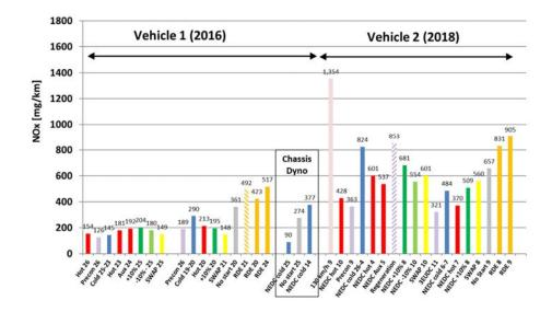
Figure 4-1: Measured NO<sub>x</sub> emissions from the first exploratory test track measurements of the two investigated Suzuki Vitaras Euro 1 diesel with engine calibration 1 The first vehicle was tested by RDW in 2016 at ambient temperatures of 20-26 °C on the test track and on the chassis dynamometer. The second vehicle was tested on the test track in 2018, at ambient temperatures of 4-11 °C.
