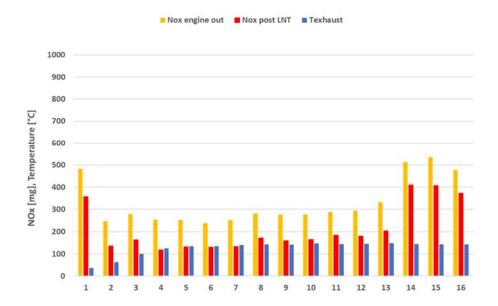
Figure 5-7:  $NO_x$  emissions per ECE cycle with engine calibration 2 in a 4\*UDC test with a cold start, start-stop not active, performed on 19-09-2018. The test was started in a conditioning room of 26 °C and was conducted on the test track of the RDW at an ambient temperature of 26 °C. Preconditioning 3\*EUDC with a warm start, conducted on 18-09-2018, with three LNT regenerations of 14 seconds in the second EUDC cycle.
