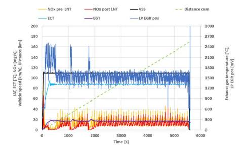
Figure 5-18: NO<sub>x</sub> and O<sub>2</sub> emissions measured at a constant speed of 110 km/h with SEMS and a vehicle with engine calibration 2, performed on 18-07-2019. The test was conducted on the test track at an ambient temperature of 26 °C. Preconditioning test 20 minutes @ 130 km/h.
