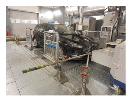
Horiba Europe GMBH performs emission tests in its laboratory in accordance with ISO 17025 standards and is certified to do this.
