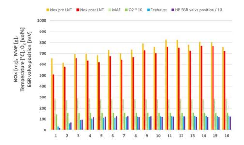
Figure 4-15: NO<sub>x</sub> emissions per ECE cycle with engine calibration 1 in a 4\*UDC test with a cold start, performed on 24-04-2018. The test was started in a conditioning room of 26°C and was conducted on the test track of the RDW at an ambient temperature of 13°C. Preconditioning 3\*EUDC with a warm start, conducted on 19-04-2019, with one LNT regeneration of 10 seconds in the first EUDC.
