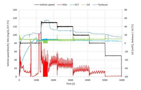
Figure 5-16:  $NO_x$  and  $O_2$  emissions measured with engine calibration 2, at a constant speed of 80, 130, 120, 100, 80 - 50 km/h (cold start) with SEMS with engine calibration 2, performed on 16-11-2018. The test was conducted on the test track at an ambient temperature of 6-10 °C. The diesel particulate filter is regenerated at 130 km/h.
