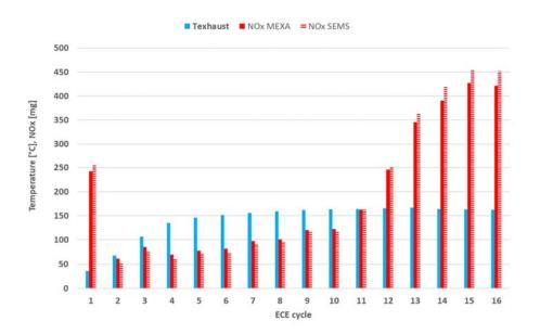
Figure 5-13: NO<sub>x</sub> measured with a chassis dynamometer analyser (MEXA) and with SEMS per ECE cycle with engine calibration 2 in a 4\*UDC test with a cold start, start-stop active, performed on 12-12-2018. The test was conducted on the chassis dynamometer at an ambient temperature of 23 °C. Preconditioning 3\*EUDC with a warm start, conducted on 11-12-2018, with 2 LNT regenerations in the second and third EUDC cycles.
