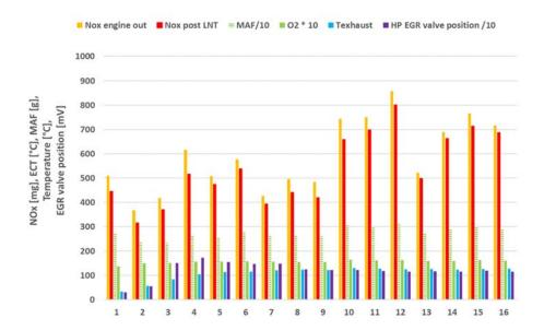
Figure 4-13: NO<sub>x</sub> emissions per ECE cycle with engine calibration 1 in a 4\*UDC test with a cold start, performed on 16-04-2018. The test was started in a conditioning room of 26°C and was conducted on the test track of the RDW at an ambient temperature of 18°C. Preconditioning 3\*EUDC with a warm start, conducted on 11-04-2018, with three LNT regenerations of 2, 15 and 14 seconds.
