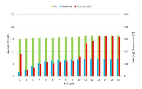
Figure 4-23: NO<sub>x</sub> emissions per ECE cycle with engine calibration 1 in a 4\*UDC test with cold start, performed on 21-08-2018. The test was driven on the chassis dynamometer with road load setting 2 and an ambient temperature of 23 °C. Preconditioning 3\*EUDC test on 17-08-2018 with a warm start with 3 LNT regenerations with a duration of 13 seconds.
