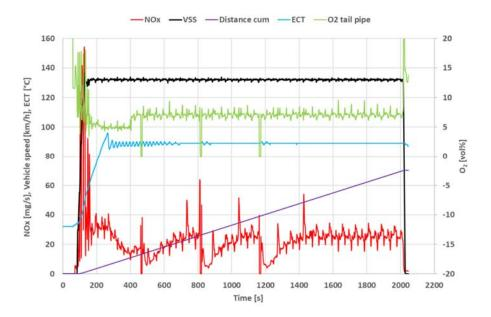
Figure 7-1:  $NO_x$  concentrations at a constant speed of 130 km/h. Due to the operation of the LNT, the  $NO_x$  emission up to t = 1500 s varies between 5 and 25 mg/s. After that, the LNT is no longer regenerated and the  $NO_x$  emission remains stable.
