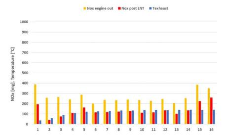
Figure 5-8: NO<sub>x</sub> emissions per ECE cycle with engine calibration 2 in a 4\*UDC test with a cold start, start-stop active, performed on 24-10-2018. The test was started in a conditioning room of 26 °C and was conducted on the test track of the RDW at an ambient temperature of 18 °C. Preconditioning 3\*EUDC test conducted on 18-10-2018, with a warm start for which no measurement data are available.
