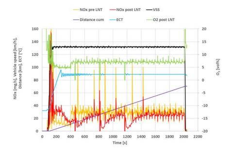
Figure 5-17:  $NO_x$  and  $O_2$  emissions measured with engine calibration 2 at a constant speed of 130 km/h after a cold start with SEMS, conducted on 31-08-2018. The test was conducted on the test track at an ambient temperature of 20-23 °C.
