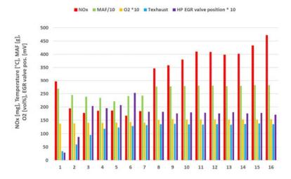
Figure 4-12: NO<sub>x</sub> emissions per ECE cycle with engine calibration 1 in a 4\*UDC test with a cold start, performed on 10-04-2018. The test was started in a conditioning room of 26°C and was conducted on the test track of the RDW at an ambient temperature of 22°C. Preconditioning 3\*EUDC with a warm start, conducted on 09-04-2018, with three LNT regenerations of 13, 13 and 5 seconds.
