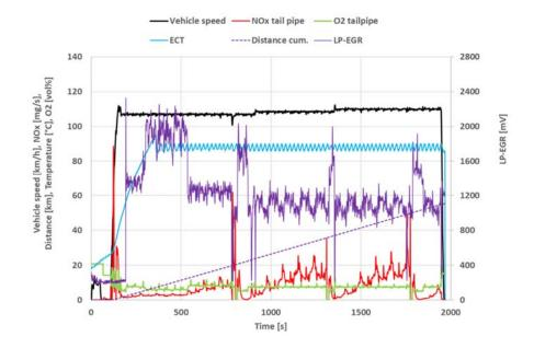
Figure 5-15:  $NO_x$  and  $O_2$  emissions measured with engine calibration 2 at a constant speed of 110 km/h (cold start) with SEMS, conducted on 17-04-2019. The test was conducted on the test track at an ambient temperature of 20 °C. The position signal of the low-pressure EGR valve is also shown.
