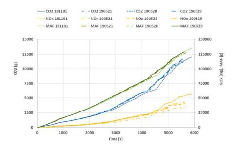
Figure 5-20: Cumulative CO<sub>2</sub> and NO<sub>x</sub> emissions measured in RDE tests with engine calibration 2.
