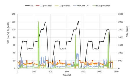
Figure 4-6: 3\*EUDC test with engine calibration 1 and warm start, conducted on 29-05-2018 on the test track, at an ambient temperature of 28 °C. The LNT is regenerated three times for 10-13 seconds. The last EUDC cycle ended after the 100 km/h part of the LNT regeneration.
