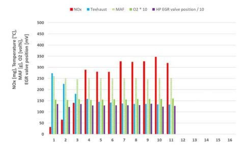
Figure 4-17: NO<sub>x</sub> emissions per ECE cycle with engine calibration 1 in a 4\*UDC test with a warm start, performed on 10-04-2018. The test was started and driven on the test track of the RDW at an ambient temperature of 22 °C. Preconditioning 10 minutes @ 120 km/h with a warm start with various LNT regenerations.
