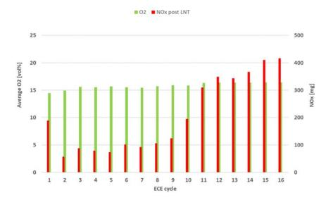
Figure 4-24: NO<sub>x</sub> emissions per ECE cycle with engine calibration 1 in a 4\*UDC test with a cold start, performed on 03-09-2018. The test was driven on the chassis dynamometer with road load setting 3 and an ambient temperature of 23 °C. Preconditioning 3\*EUDC test on 02-09-2018 with a warm start for which no measurement data are available.
