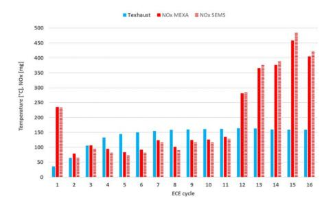
Figure 5-12: NO<sub>x</sub> measured with a chassis dynamometer analyser (MEXA) and with SEMS per ECE cycle with engine calibration 2 in a 4\*UDC test with a cold start, start-stop active, performed on 11-12-2018. The test was conducted on the chassis dynamometer at an ambient temperature of 23 °C. Preconditioning 3\*EUDC with a warm start, conducted on 10-12-2018, with 3 LNT regenerations in the second and third EUDC cycles.
