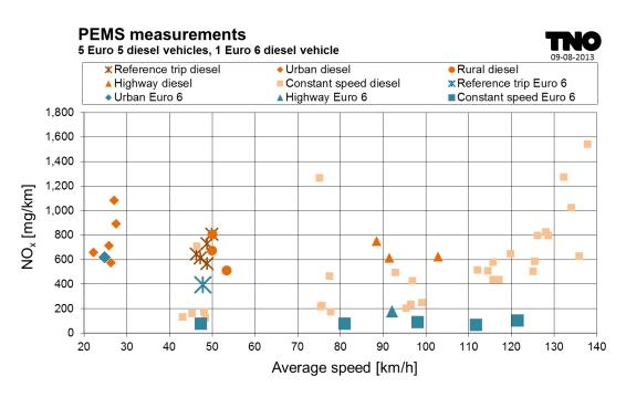
Figure 17: Absolute PEMS results for Euro 5 vehicles and vehicle E6
