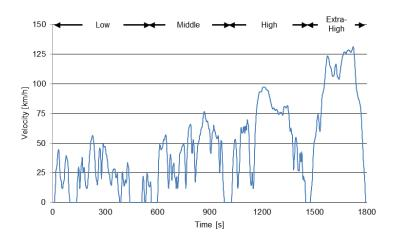
Figure 5: WLTC\_v5 (Worldwide harmonized Light duty driving Test Cycle)
