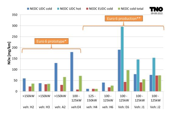
Figure 15: NO<sub>x</sub> emissions per phase in the NEDC
