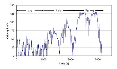
Figure 4: CADC (Common Artemis Driving Cycle)
