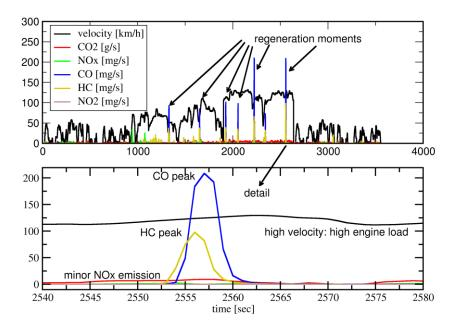
Figure 22: Typical regeneration moments at high velocities. A peak of CO and HC with limited NO<sub>x</sub> emissions.
