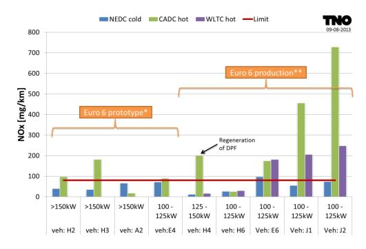
Figure 14: NO<sub>x</sub> emissions per driving cycle
