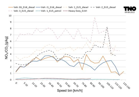
Figure 19: PEMS results binned in NO<sub>x</sub> over CO<sub>2</sub>
