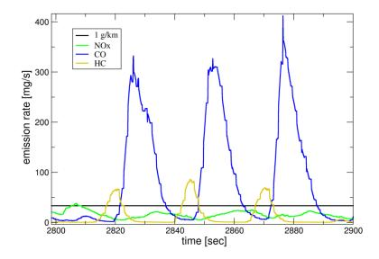
Figure 23: LNT emission control during motorway driving yielding a fast succession of regenerations with still substantial  $NO_x$  emissions.
