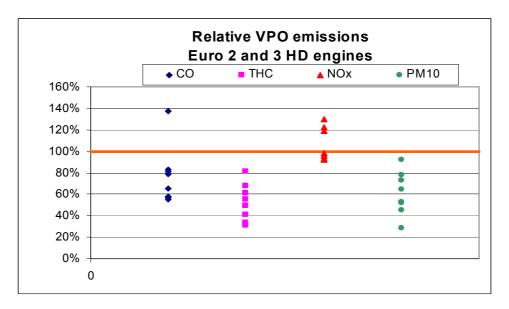
Figure 5.15 Exhaust emissions of HD engines on VPO [Bünger 2007], [Hausberger 2007], [TNO2007b], [Lenaers 2008]
