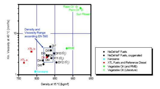
Figure 6.3 Kinematic viscosity and density of different fuels (EN590 window shows the boundaries for diesel) [Fricke 2007]
