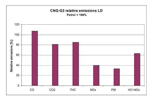
Figure 5.3 Relative emissions CNG Euro III LD-vehicle [TNO 2003b]
