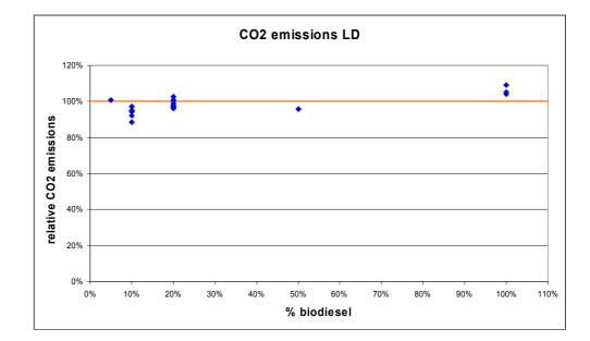
Figure 5.14 CO<sub>2</sub> emissions from LD vehicles on biodiesel (blends)
