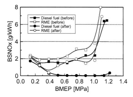
Figure 6.10 Emissions of 100% RME compared to reference diesel on NO<sub>x</sub> emissions before and after catalyst of a turbocharged CI engine with variable EGR and a DPNR aftertreatment system [Kawano 2007]
