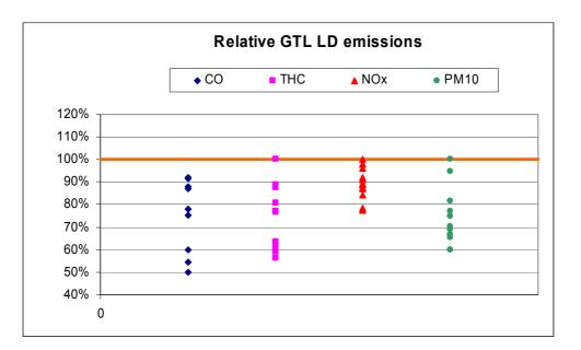
Figure 5.18 Exhaust emissions from LD vehicles on GTL [Alleman 2003], [Kitano 2007], [Schaberg 2005]
