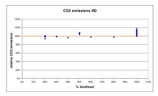
Figure 5.13 CO<sub>2</sub> emissions from HD engines on biodiesel (blends)
