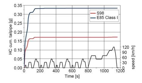
Figure 6.8 Cumulative HC emissions over the NEDC Cycle for a vehicle running on premium petrol (S98) and on Class 1 E85 [Benninger 2007]
