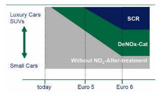
Figure 3.3 Exhaust aftertreatment technologies for passenger cars
