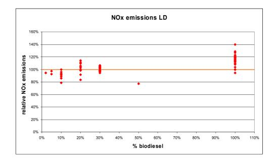
Figure 5.10 NO<sub>x</sub> emissions from LD vehicles on biodiesel (blends)
