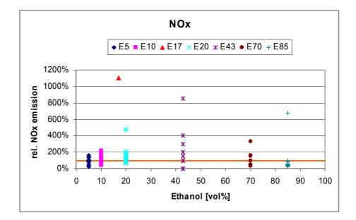
Figure 5.22 NO<sub>x</sub> emissions from LD vehicles on ethanol blends
