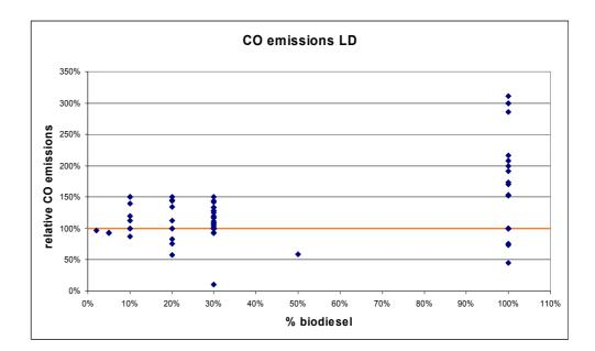
Figure 5.6 CO emissions from LD vehicles on biodiesel (blends)
