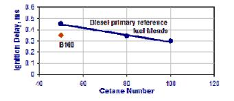
Figure 6.2 Effect of cetane number for three primary reference fuel blends and B100 [Dieselnet 2007]
