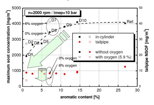
Figure 6.4 Maximum soot concentration (in-cylinder and at the tailpipe) as a function of aromatic and oxygen content in the fuel [Fricke 2007][Pischinger 2007]
