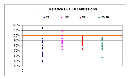
Figure 5.17 Exhaust emissions from HD engines on GTL [Alleman 2003], [Clark 2005], [Krahl 2005], [Thompson 2004],
