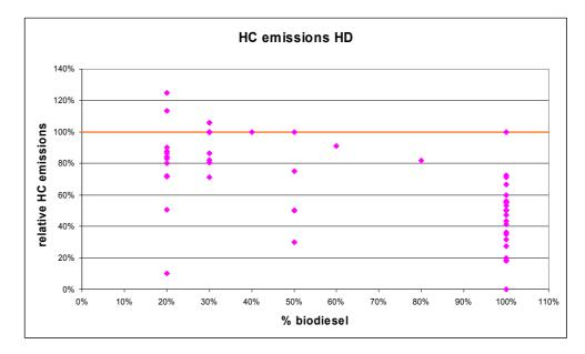
Figure 5.7 HC emissions from HD engines on biodiesel (blends)
