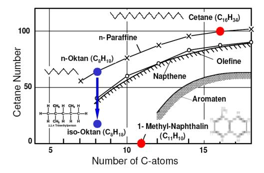
Figure 6.1 Cetane number as a function of C atom number for different kinds of molecule structures [Fricke 2007][Pischinger 2007]
