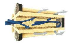
Figure 3.2 Diesel particulate wall flow filter (DPF)
