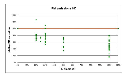
Figure 5.11 PM emissions from HD engines on biodiesel (blends)
