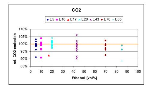
Figure 5.24 CO<sub>2</sub> emissions from LD vehicles on ethanol blends
