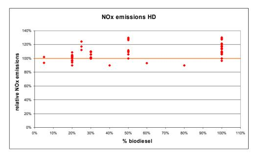
Figure 5.9 NO<sub>x</sub> emissions from HD engines on biodiesel (blends)
