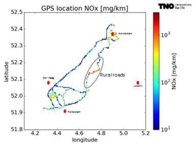
Figure 6: Emission measurement results of a modern Euro-6c diesel passenger car plotted on a real-world trip. The car showed good performance during driving on motorways with speed limits in force and expectedly higher emissions in urban areas. Emission performance during rural driving varied strongly. Source: TNO report: 'TNO 2016 R11227: Assessment of the strengths and weaknesses of the new Real Driving Emissions (RDE) test procedure'.
