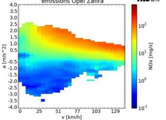
Figure 7: Typical emission map of a modern Euro 6 diesel passenger car, based on on-road emission measurements. Source: TNO 2016 R11177 "NO<sub>x</sub> emissions of fifteen Euro 6 diesel cars: Results of the Dutch road vehicle emission testing program 2016", Heijne et.al.
