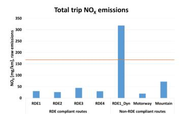
Figure 1: Emissions over different RDE compliant and non-compliant trips as measures by the JRC². The measured vehicle is an Euro 6dTemp equipped with EGR, DOC, SCR and DPF technology.
