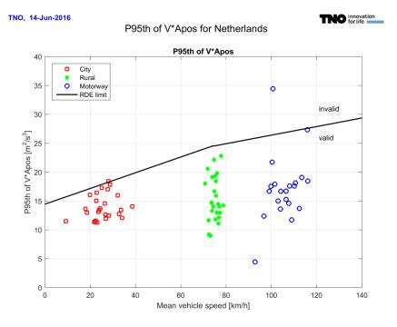
Figure 4:  $v * a_{pos}$  values for typical driving behaviour in the Netherlands per road section <sup>1</sup>
