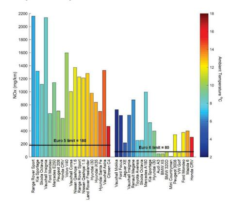
Figure 5: NO<sub>x</sub> results from the recently published UK Vehicle Testing Programme. <sup>5</sup> Track test results plotted in order of increasing ambient temperature.
