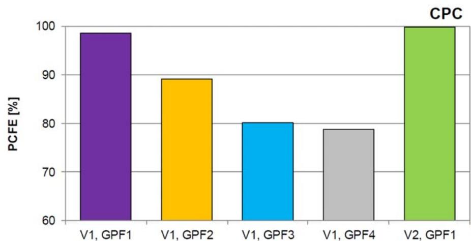
Figure 13: PN emission filtration efficiencies of four different GPFs in WLTC tests, GPF 1 was tested at two vehicle types (source GasOMeP project, Switzerland).
