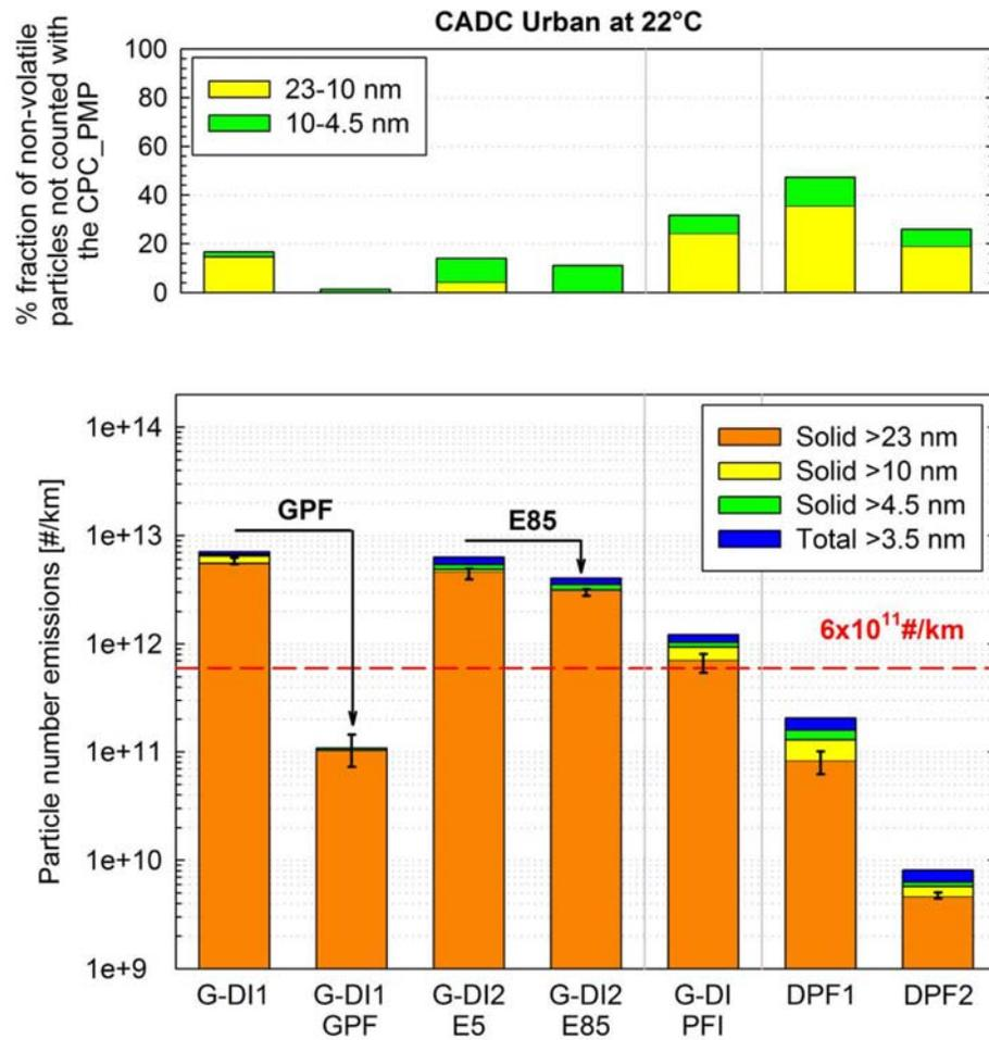
Figure 18: Particle number emission rates of the different vehicles tested over the urban phase of the CADC (bottom chart) and fraction of sub-23nm non-volatile particle counts not detected with the PMP CPC (top chart). Explanations as in Figure 18.
