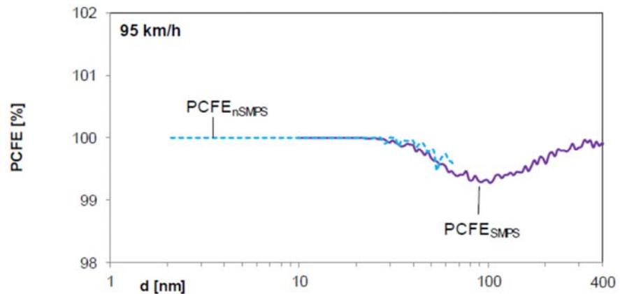
Figure 15: PN emission filtration efficiencies over the total particle size range of GDI vehicle 1 with GPF1 @ 95 km/h (source GasOMeP project, Switzerland)
