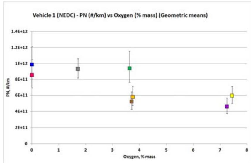
Figure 4: PN emissions of a Euro 4 GDI vehicle. with different fuels (source CONCAWE).
