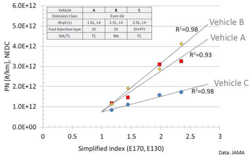
Figure 8: Different fuel compositions (expressed with the simplified PM index) and NEDC PN emissions (Source JAMA) of GDI and PFI engines. Source JAMA.
