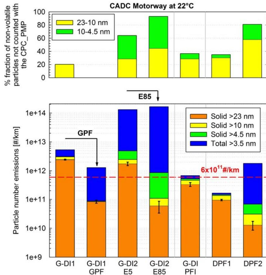
Figure 20: Particle number emission rates of the different vehicles tested over the motorway phase of the CADC (bottom panel) and fraction of sub-23nm non-volatile particle counts not detected with the PMP CPC (top panel). Explanations as in Figure 18.
