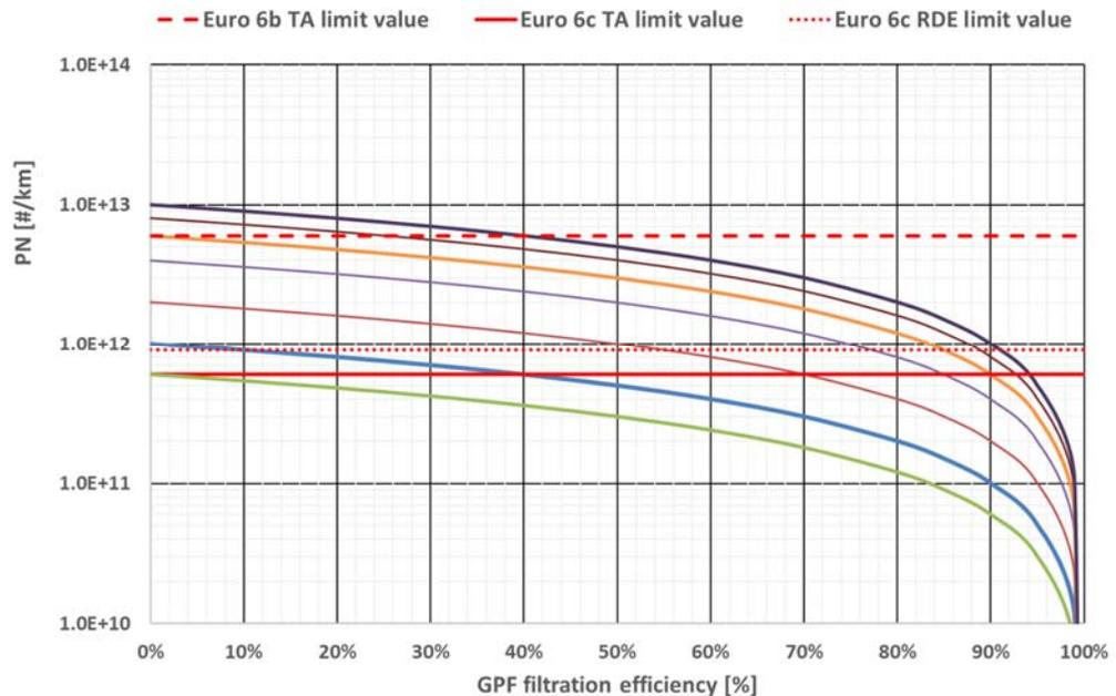
Figure 11: Sketch of PN tail pipe emissions of vehicles with different PN emissions and different GPF filtration efficiencies (1).
