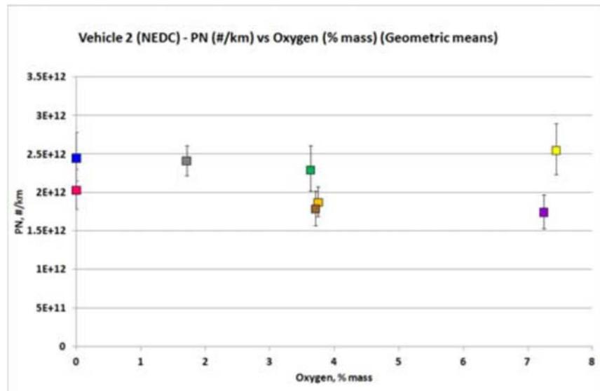
Figure 5: PN emissions of a Euro 5 GDI vehicle. with different fuels (source CONCAWE).
