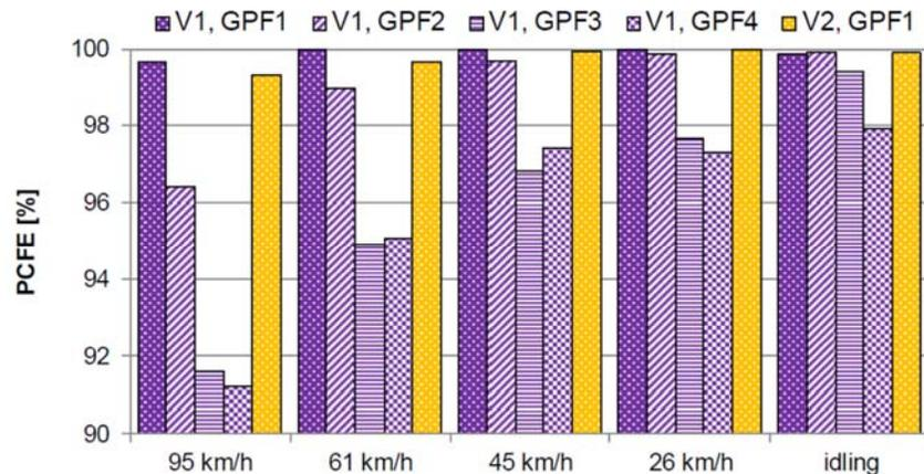
Figure 14: PN emission filtration efficiencies of four different GPFs at constant velocities, GPF 1 was tested at two vehicle types (source GasOMeP project, Switzerland).
