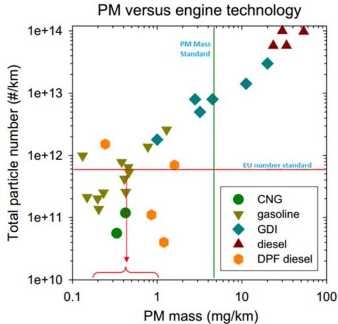
Figure 6: Particle Number vs. Particle Mass for various LDV engine technologies (source Maricq M., How are emissions of nuclei mode particles affected by new PM control technologies and fuels?, Ford Motor Company, Health Effects Institute Annual Conference, 2009).
