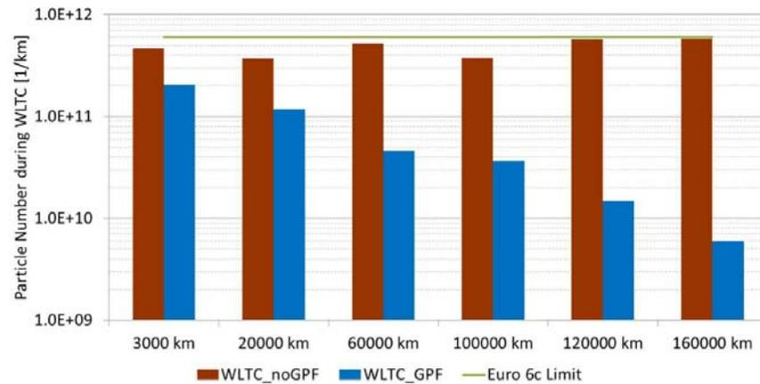
Figure 22: Tailpipe PN emissions in WLTC tests with and without underfloor catalysed GPF on a 1.8 l GDI Euro 5 engine measured at different mileages (source NGK).
