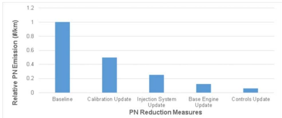
Figure 10: Impact of PN control measures on PN reduction (source GM, September 2016).
