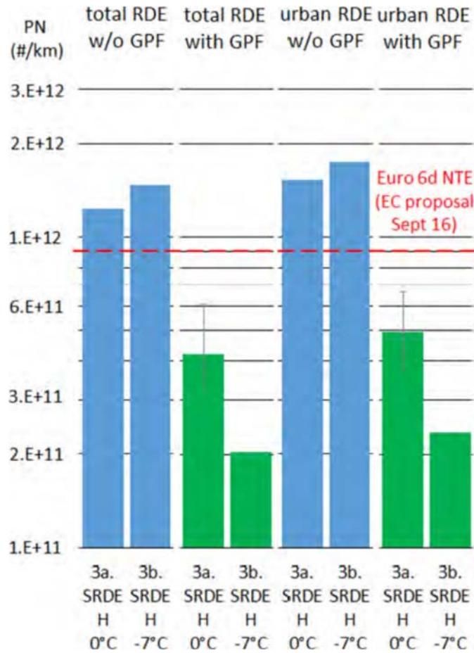
Figure 7: Total and urban RDE PN emissions measured on the dyno at low ambient temperatures (source AECC).
