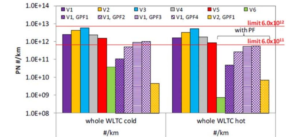
Figure 12: WLTC PN emissions of 6 GDI vehicles. On vehicle 1 and 2 four different GPFs were tested (source GasOMeP project, Switzerland).
