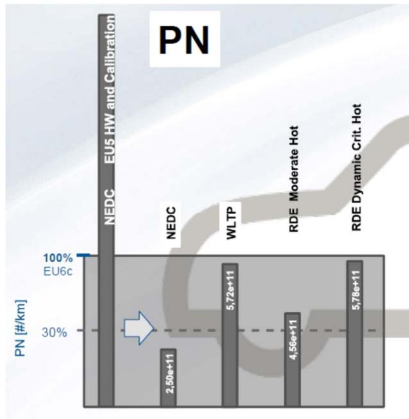
Figure 9: PN emissions of a 1600 kg SUV with 1.0 ltr GDI engine (source AVL)
