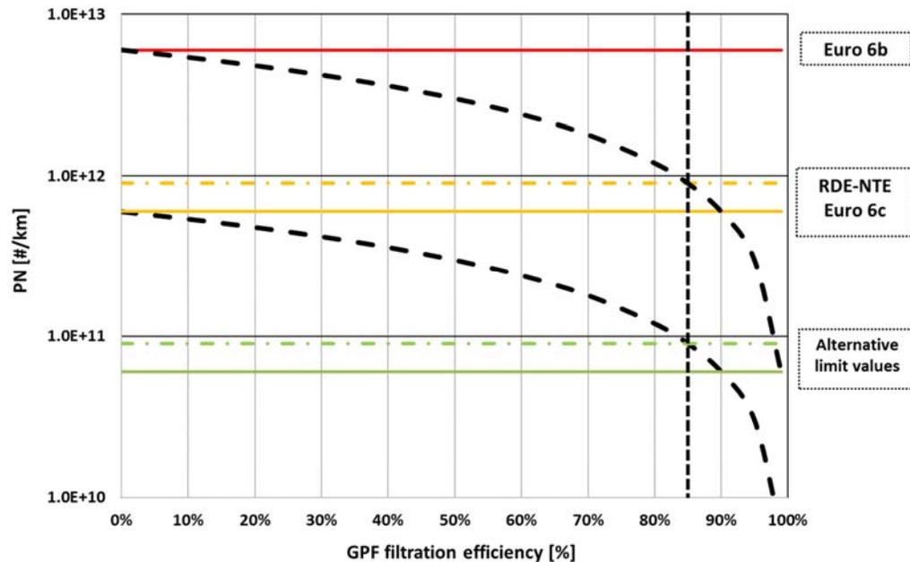
Figure 24: Simulation of PN tail pipe emissions of vehicles with different PN emissions and different GPF filtration efficiencies (2).
