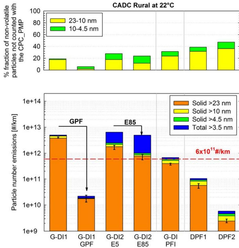
Figure 19: Particle number emission rates of the different vehicles tested over the rural phase of the CADC (bottom chart) and fraction of sub-23nm non-volatile particle counts not detected with the PMP CPC (top chart). Explanations as in Figure 18.
