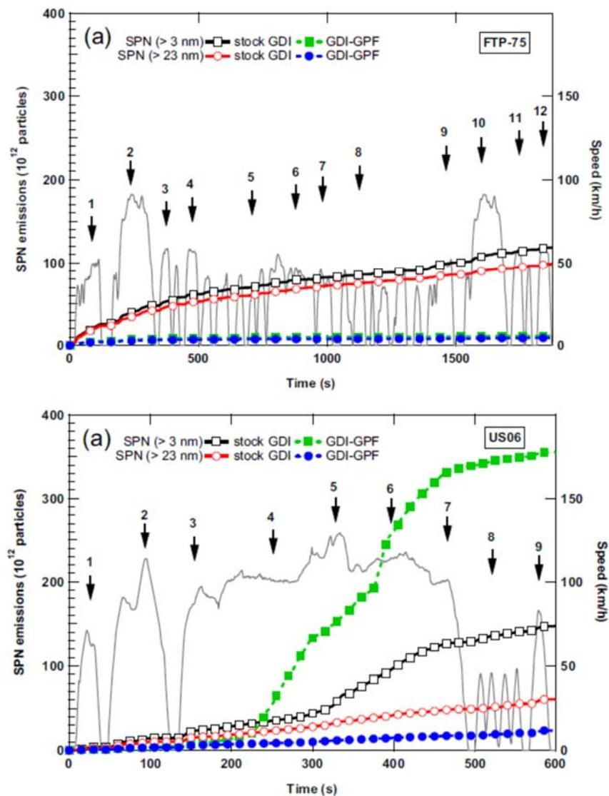
Figure 21: FTP-75 and US06 PN emissions ( $>23$  nm and  $>3$  nm) of a Ford Focus 2.0 GDI with and w/o GPF (source Chan et al.)
