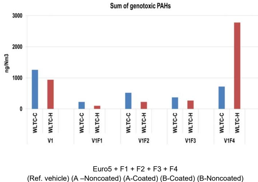
Figure 16: Genotoxic PAH emissions of a Euro 5 GDI vehicle tested with four different GPF types.
