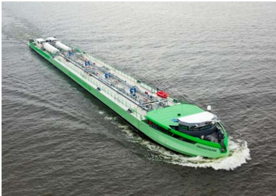
Figure 11: Tanker “Greenstream” with LNG-electric propulsion [IWN2013]
