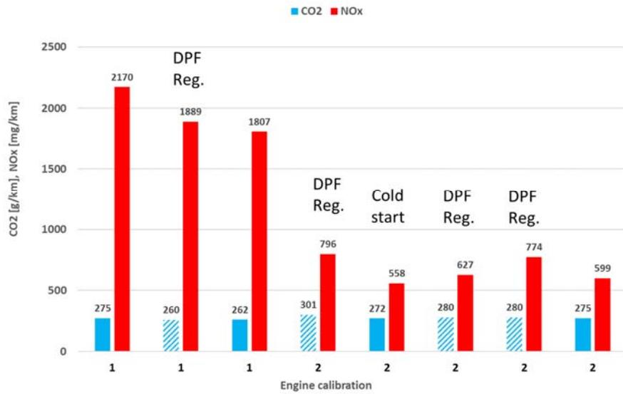
Figure 4-33: CO<sub>2</sub> and NO<sub>x</sub> results from RDE tests of the Jeep Grand Cherokee Euro 5a diesel conducted in Lelystad with two different engine calibrations
