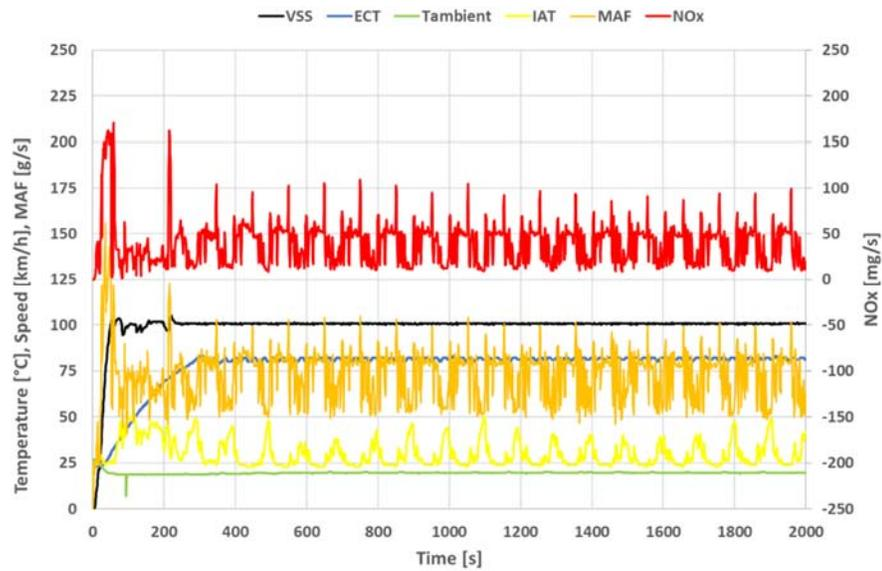
Figure 4-16: NO<sub>x</sub> emissions during a cold start with engine calibration 1 and a constant speed of 100 km/h. During the period in which the coolant temperature is rising (ECT is 20 - 80 °C), the NO<sub>x</sub> emission varies. The NO<sub>x</sub> emission of a warmed up engine (ECT is 80 °C) fluctuates between 10 and 50 mg/s.
