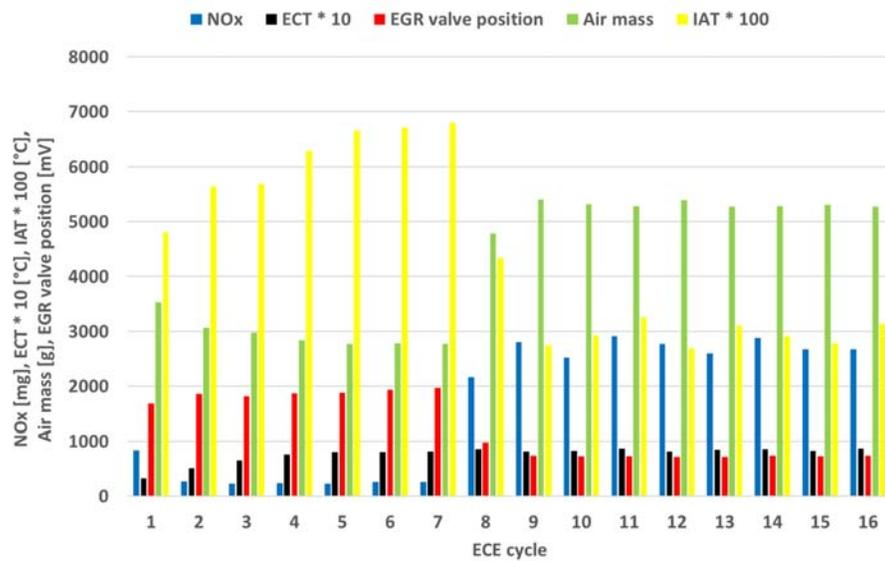
Figure 4-10: NO<sub>x</sub> emission, air consumption and average ECT, IAT and position signal of the EGR valve per ECE cycle of a 4\*UDC test with engine calibration C1 and cold start, performed on 03-04-2018. The test started in a conditioning room of 25 °C and was conducted on the test track of the RDW with an ambient temperature of 18-20 °C. Preconditioning 3\*EUDC with hot start.
