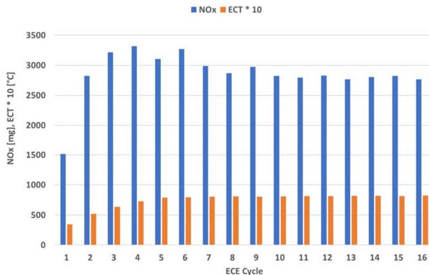
Figure 4-8: NO<sub>x</sub> emissions per ECE cycle of a 1\*UDC test with engine calibration C1 and a cold start, performed on 28-03-2018. The test started in a conditioning room of 26 °C and was conducted on the test track of the RDW with an ambient temperature of 10 °C. Preconditioning 3\*EUDC with hot start.
