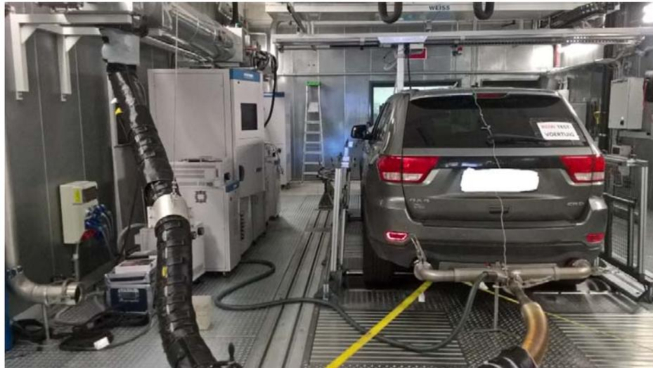
Figure 3-1: Dynamometer with measurement equipment for performing an emissions test
