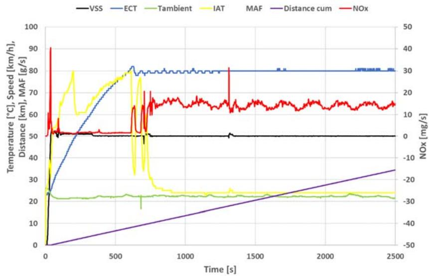
Figure 4-15: NO<sub>x</sub> emissions during a cold start with engine calibration C1 and a constant speed of 50 km/h. During the period in which the coolant temperature is rising (ECT is 20 - 80 °C), the NO<sub>x</sub> emissions are less than 2 mg/s. The NO<sub>x</sub> emission of the warmed up engine (ECT is 80 °C) is 11 – 17 mg/s.
