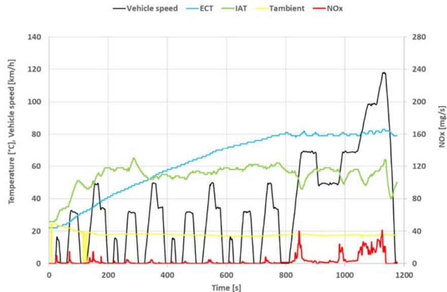
Figure 4-29: NEDC test with engine calibration C2 and cold start of 18-10-2018 on the test track, at an ambient temperature of 18 °C. The inlet temperature was 50-60 °C for almost the entire test, indicating an active EGR system. CO<sub>2</sub> = 312 g/km and NO<sub>x</sub> = 376 mg/km.
