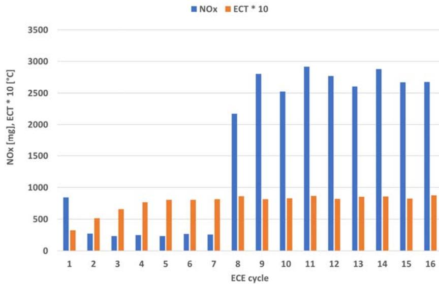
Figure 4-9: NO<sub>x</sub> emissions per ECE cycle of a 4\*UDC test with engine calibration C1 and a cold start, performed on 03-04-2018. The test was started in a conditioning room of 25 °C and was conducted on the test track of the RDW with an ambient temperature of 18-20 °C. Preconditioning 3\*EUDC with hot start.
