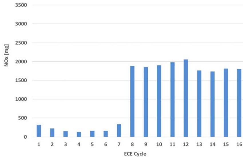
Figure 4-21: NO<sub>x</sub> emissions per ECE cycle of a UDC test with cold start and engine calibration C1, performed on 24-08-2018 on the dynamometer with adjusted settings (RL2) and an ambient temperature of 23 °C. Preconditioning 3\*EUDC with hot start.
