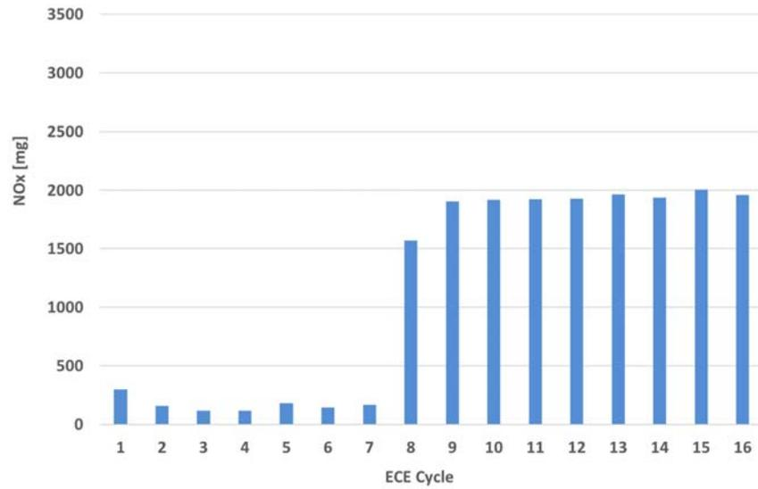
Figure 4-20: NO<sub>x</sub> emissions per ECE cycle of a UDC test with cold start and engine calibration C1, performed on 21-08-2018 on the dynamometer with adjusted settings (RL2) and an ambient temperature of 23 °C. Preconditioning 3\*EUDC with hot start.
