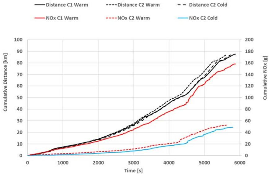
Figure 4-34: Cumulative NO<sub>x</sub> results from RDE tests of the Jeep Grand Cherokee Euro 5 diesel conducted in Lelystad with two different engine calibrations
