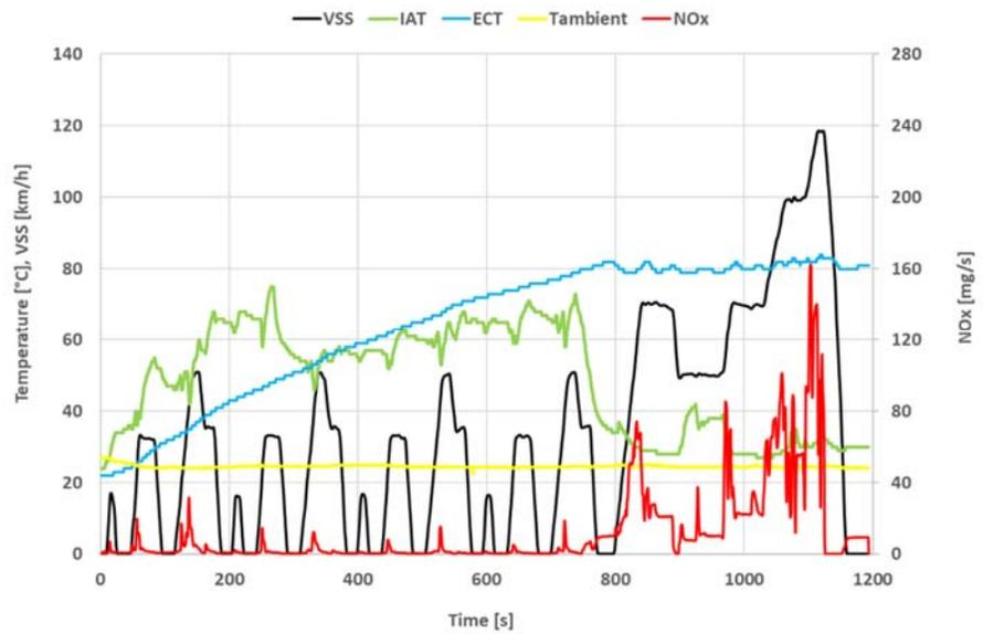
Figure 4-5: NEDC test with engine calibration 1 and cold start on 22-05-2018 on the test track. After 750 seconds, the temperature in the engine inlet (IAT) drops and the NO<sub>x</sub> emissions rise substantially.
