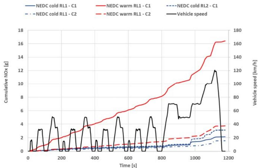
Figure 4-26: Cumulative representation of the NO<sub>x</sub> emissions from NEDC tests with cold and hot starts (c and h), two different driving resistance curves (RL1 and RL2), and two different engine calibrations (C1 & C2)
