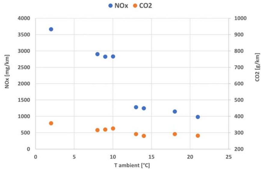
Figure 4-4: NO<sub>x</sub> and CO<sub>2</sub> emissions measured on the test track with engine calibration 1 at different ambient temperatures
