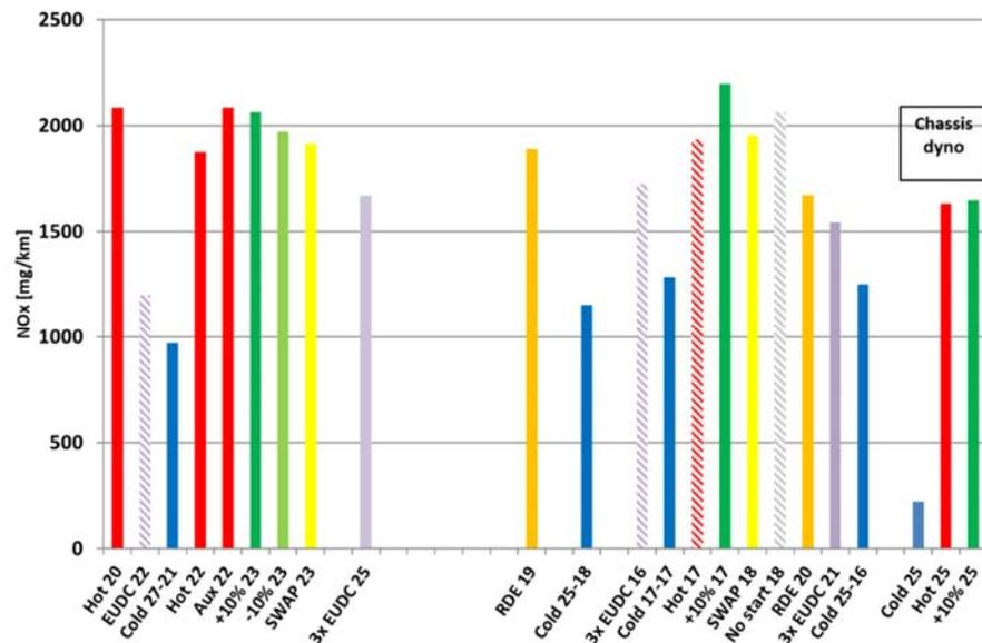
Figure 1-1: NO<sub>x</sub> test results from the first exploratory measurements of a Jeep Grand Cherokee Euro 5a diesel in 2017. Source: [RDW 2017].
