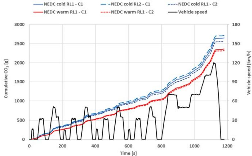
Figure 4-27: Cumulative representation of CO<sub>2</sub> emissions from NEDC tests with cold and hot starts (c & h), two different driving resistance curves (RL1 and RL2) and two different engine calibrations (C1 & C2).
