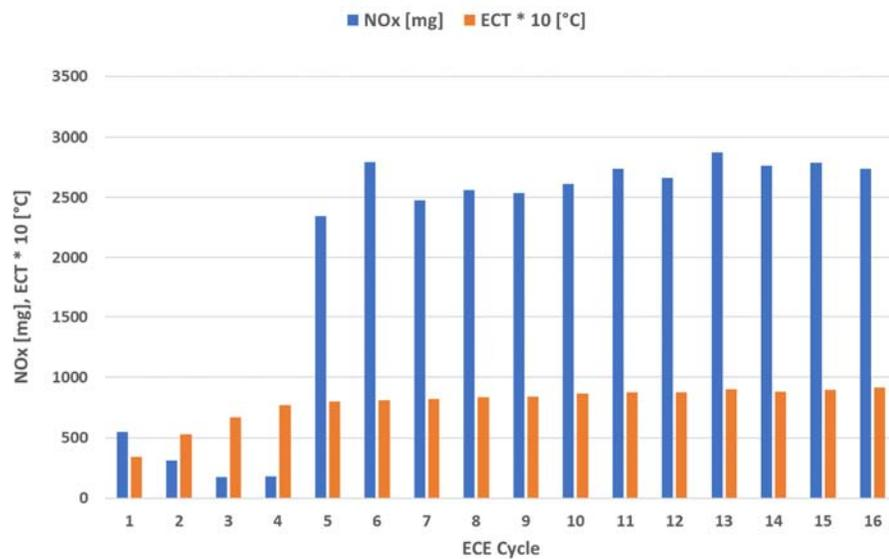
Figure 4-12: NO<sub>x</sub> emissions per ECE cycle of a 4\*UDC test with engine calibration C1 and cold start, performed on 19-04-2018. The test was started in a conditioning room of 25 °C and was conducted on the test track of the RDW with an ambient temperature of 27 °C. Preconditioning 3\*EUDC with hot start.
