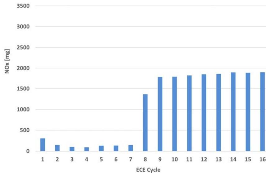
Figure 4-19: NO<sub>x</sub> emissions per ECE cycle of a UDC test with cold engine start and engine calibration C1, performed on 23-08-2018 on the dynamometer with settings according to manufacturer's specifications (RL1) and an ambient temperature of 23 °C. Preconditioning 3\*EUDC with a hot start.
