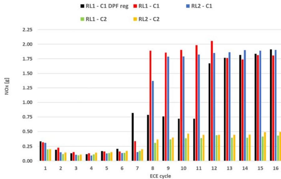
Figure 4-28: NO<sub>x</sub> emissions per ECE cycle of UDC cold start tests, performed on the dynamometer with two engine calibrations (C1 & C2), two dynamometer settings (RL1, RL2), at an ambient temperature of 23 °C. Preconditioning 3\* EUDC with hot start. A soot filter regeneration was carried out in the first test (black).
