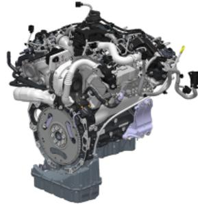
The 3.0L V6 Diesel Engine with common-rail direct injection is built at VM Motori engines plant in Cento Italy. The main engine features are CGI block, dual overhead camshafts chain driven, central injectors and four valves per cylinder.
