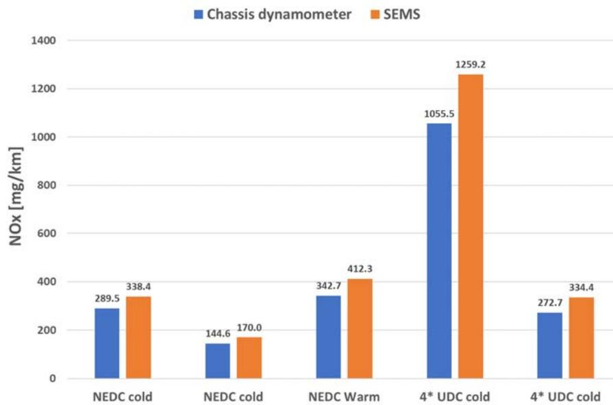
Figure 4-25: NO<sub>x</sub> emissions from five dynamometer tests measured with the dynamometer (chassis dynamometer) equipment and with the SEMS
