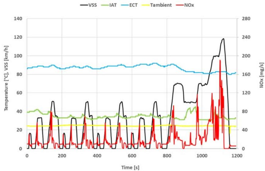
Figure 4-7: NEDC test with engine calibration 1 and cold start on 22-05-2018 on the test track. The temperature in the engine inlet (IAT) is 30 - 45 °C and relatively constant. The NO<sub>x</sub> emissions are substantially higher in the first 780 seconds in comparison to the NEDC cold start test. This is possibly caused by the (partial) shutdown of the EGR system.
