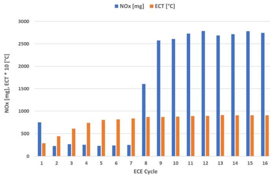
Figure 4-14: NO<sub>x</sub> emissions per ECE cycle of a 4\*UDC test with engine calibration C1 and cold start, performed on 08-05-2018. The test was started in a conditioning room of 27 °C and was conducted on the test track of the RDW with an ambient temperature of 27 °C. Preconditioning 3\*EUDC with hot start.
