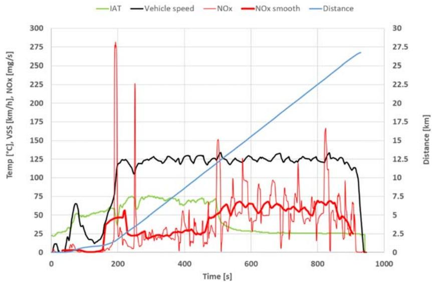
Figure 4-30: Test at a constant speed of 125 km/h with engine calibration C2 and a cold start of 23-10-2018 on the test track. The inlet temperature at 500 seconds is around 70 °C. The inlet temperature then drops to 25 °C and the NO<sub>x</sub> emissions increase from approx. 25 to 50-65 mg/s. This indicates a reduction in the added quantity of EGR.
