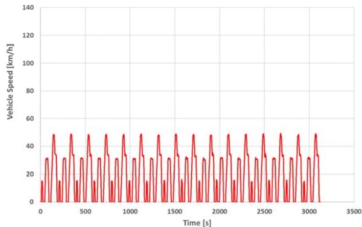
Figure 2-5: 4\*UDC test cycles, 16 kilometres in total
