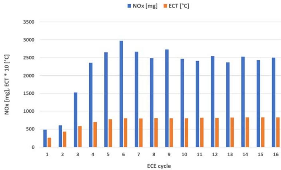
Figure 4-13: NO<sub>x</sub> emissions per ECE cycle of a 4\*UDC test with engine calibration C1 and cold start, performed on 24-04-2018. The test was started in a conditioning room of 26 °C and was conducted on the test track of the RDW with an ambient temperature of 14 °C. Preconditioning 3\*EUDC with hot start.
