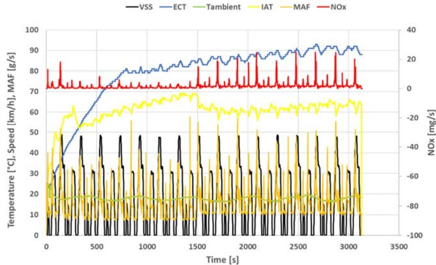
Figure 4-32: 4\*UDC test with a cold start and engine calibration C2, performed on 24-10-2018. The test was started in a conditioning room of 25 °C and was conducted on the test track of the RDW with an ambient temperature of 18 °C. Preconditioning 3\* EUDC with hot start. After 1500 seconds, the inlet temperature drops from 70 to 60 °C and the NO<sub>x</sub> emissions increase.
