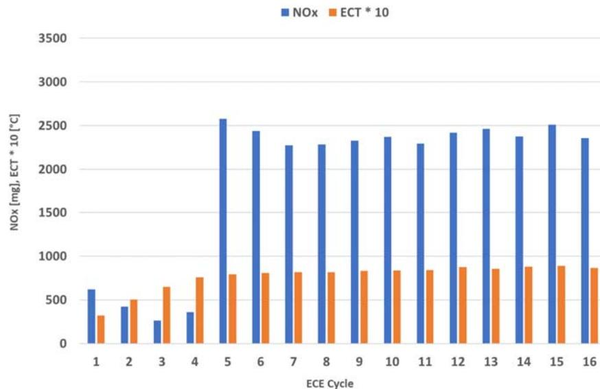
Figure 4-23: NO<sub>x</sub> emissions per ECE cycle of a 4\*UDC test with cold start and engine calibration C1, performed on 25-05-2018. The test was started in a conditioning room of 25 °C and was conducted on the test track of the RDW with an ambient temperature of 25 °C. The SEMS and the driver aid were connected to an external power supply. Preconditioning 3\*EUDC with hot start.
