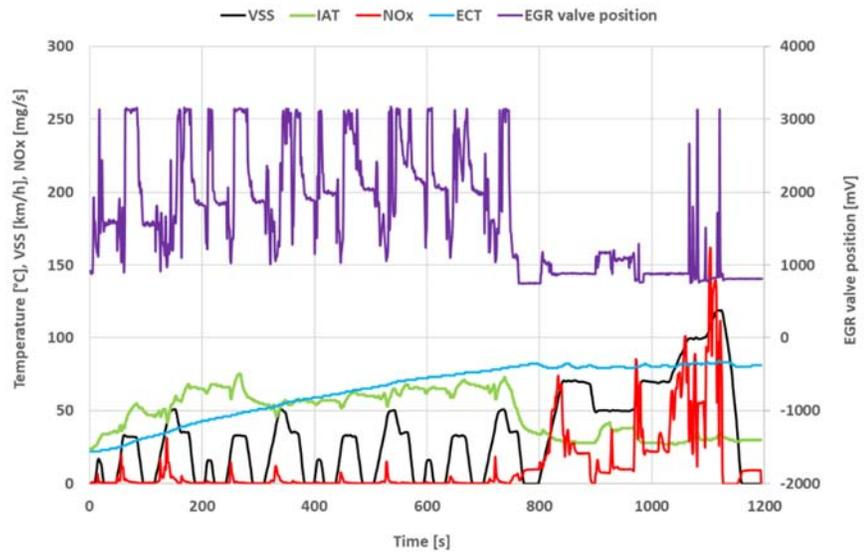
Figure 4-6: NEDC test with engine calibration 1 and cold start on 22-05-2018 on the test track. After 750 seconds, the temperature in the engine inlet (IAT) drops and the NO<sub>x</sub> emissions rise substantially. This is possibly caused by the (partial) shutdown of the EGR system. The position signal of the EGR valve varies between 1000 and 3000 mV during the first 750 seconds. After 750 seconds, The EGR valve shows a relatively stable position signal (usually <1000 mV).
