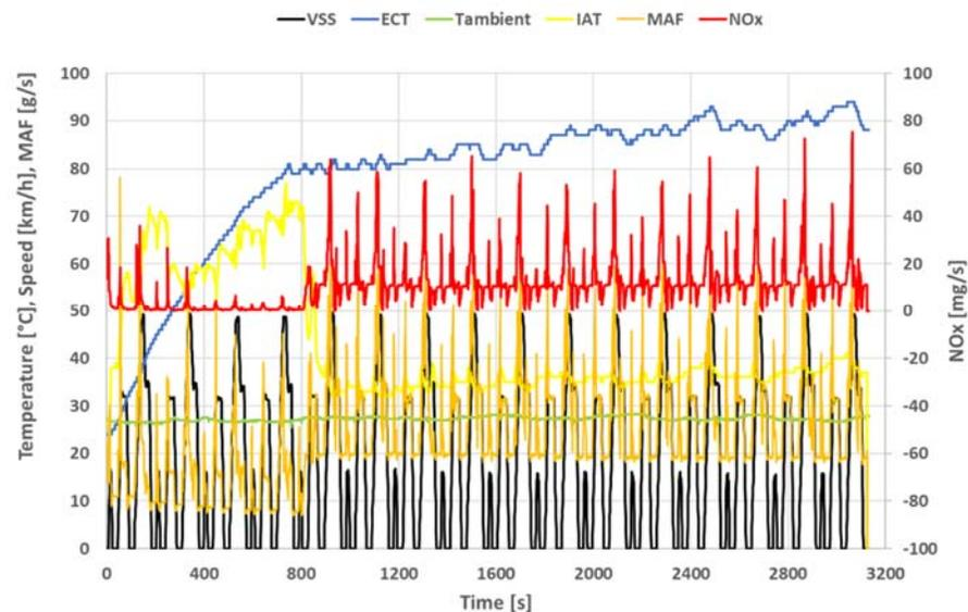
Figure 4-17: Diverse parameters of a 4\*UDC test with a cold start and engine calibration C1, performed on 19-04-2018. The test started in a conditioning room of 25 °C and was conducted on the RDW test track with an ambient temperature of 27 °C.
