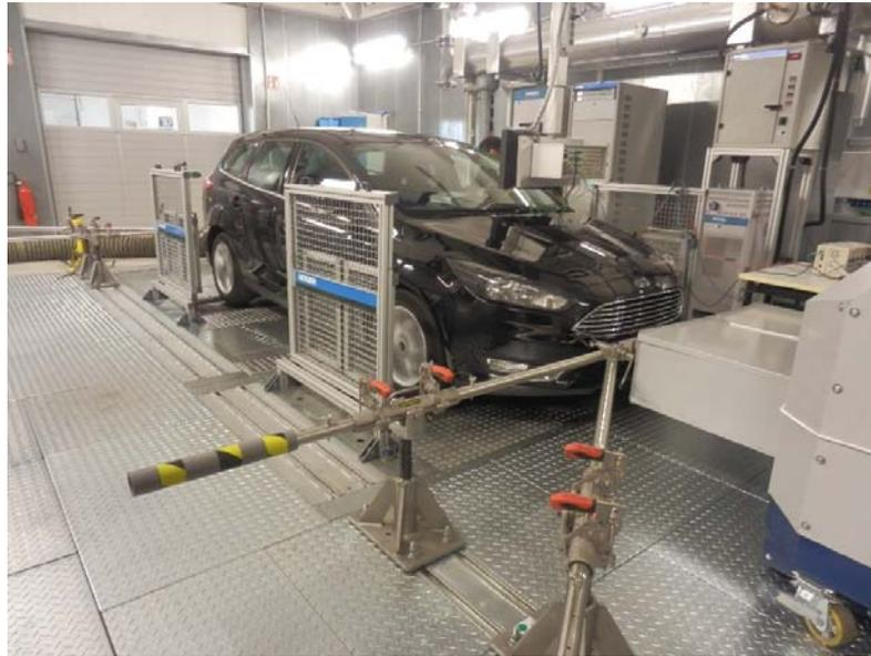
Horiba Europe GMBH performs emission tests in its laboratory in accordance with ISO 17025 standards and is certified to do this.
