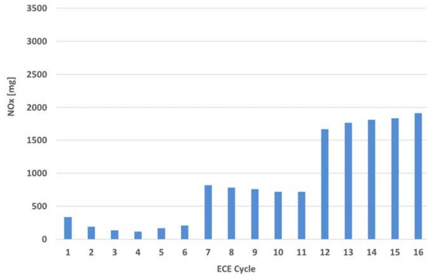
Figure 4-18: NO<sub>x</sub> emissions per ECE cycle of a UDC test with a cold start and engine calibration C1, performed on 16-08-2018 on the dynamometer with settings according to manufacturer's specifications (RL1) and an ambient temperature of 23 °C. Preconditioning NEDC with hot start.
