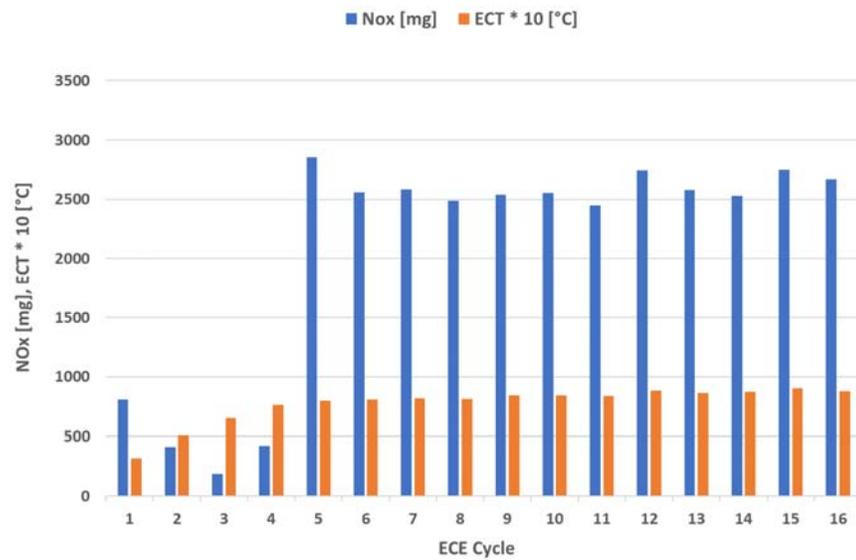
Figure 4-11: NO<sub>x</sub> emissions per ECE cycle of a 4\*UDC test with engine calibration C1 and cold start, performed on 09-04-2018. The test started in a conditioning room of 25 °C and was conducted on the test track of the RDW with an ambient temperature of 20 °C. Preconditioning 3\*EUDC with hot start.
