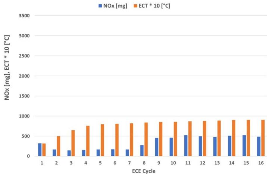
Figure 4-31: NO<sub>x</sub> emissions per ECE cycle with engine calibration C2 in a 4\*UDC test with cold start, performed on 24-10-2018. The test was started in a conditioning room of 25 °C and was conducted on the test track of the RDW with an ambient temperature of 18 °C. Preconditioning 3\*EUDC with hot start.
