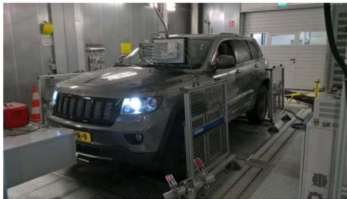
Figure 2-1: A Jeep Grand Cherokee on the dynamometer
