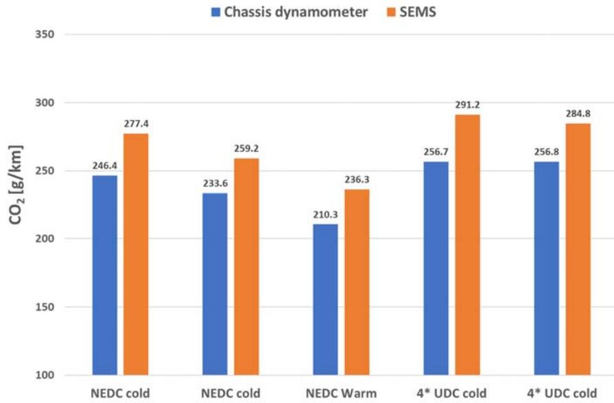
Figure 4-24: CO<sub>2</sub> emissions from different dynamometer tests measured with the dynamometer (chassis dynamometer) equipment and with the SEMS
