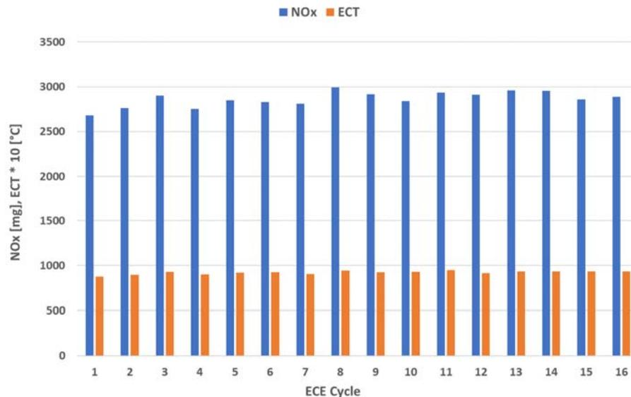
Figure 4-22: NO<sub>x</sub> emissions per ECE cycle of a 4\*UDC test with cold start and engine calibration C1, performed on 19-04-2018. The test was done on the test track of the RDW with an ambient temperature of 28 - 30 °C. Preconditioning 4\*UDC with a cold start.
